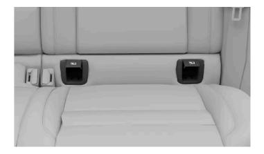
The ISOFIX<sup>[1]</sup> attachment points for the rear seats are located behind covers in the lower part of the backrest on the outer rear seats. The covers need to be lifted to access the anchor points behind them.
