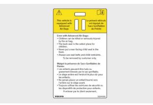
On new vehicles, this label is located in front of the dashboard on the front passenger side.
