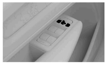
Controls for adjusting the door mirrors
