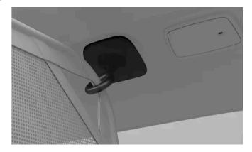
Fasten the lower corners of the net to the load-retaining eyelets behind the seats. 6
