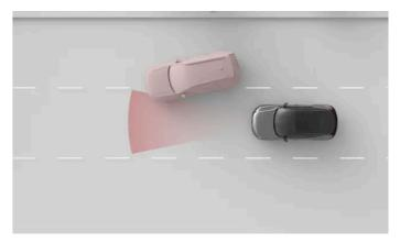
The front radar's detection zone has a limited width. If you get cut off by another vehicle, detection can occur relatively late, causing your vehicle to respond suddenly.
