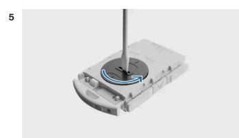
Using a suitable tool, such as a screwdriver or a coin, turn the battery cover counter-clockwise to release it.
