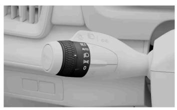
The passing beam symbol on the rotating ring on the left-hand stalk
