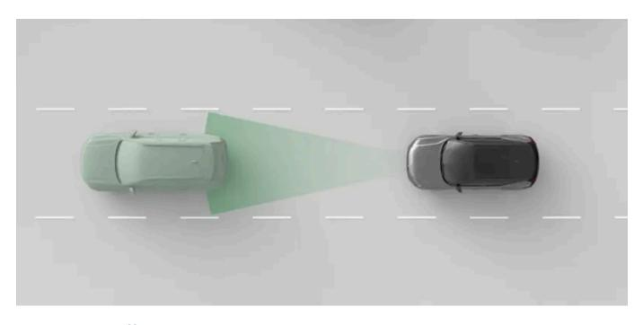
Adaptive cruise control<sup>[1]</sup> can support you with maintaining a set speed. When driving with adaptive cruise control active, you select a target speed. The vehicle then manages acceleration and braking to meet that target while also adapting to surrounding traffic.
