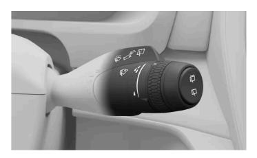
You control the wipers and washers using the right-hand steering wheel stalk.
