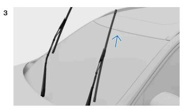
Press the button on the wiper arm and remove the wiper blade by pulling it upward.
