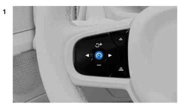
When it's safe to do so, press the adaptive cruise control button (S) on the steering wheel.
