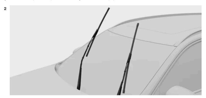
1 Activate the wiper service position via settings in the center display.
