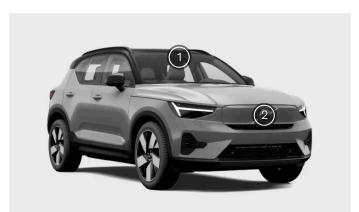
$\overbrace{1}$  The top center of the windshield houses a front-facing camera.
