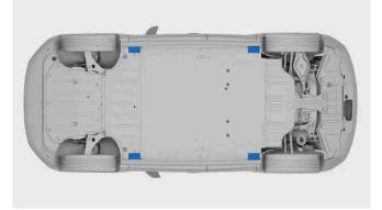
There are two jacking points on each side of the vehicle.
