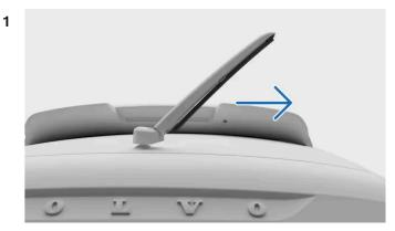
Grasp the center of the wiper arm and lift it up and away from the rear windshield. You may feel some resistance halfway – this is the lock position. You need to pull the wiper arm past the lock position so that it doesn't fall back onto the windshield
