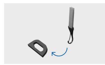
Fastening tether to lower tether attachment point
