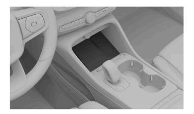
To use the wireless charger, your device should be certified to the Qi wireless charging standard. Also make sure that wireless charging is enabled on both the device<sup>[1]</sup> and on the charger itself. You can enable the charger in the center display.
