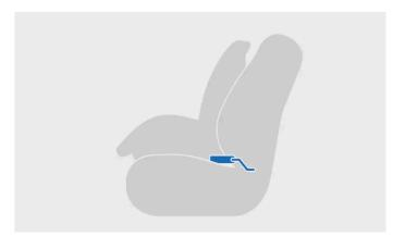
Child restraint installed using ISOFIX<sup>[1]</sup>
