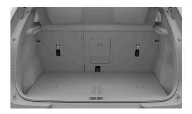
The top tether attachment point locations for the outer rear seats are indicated by the top tether symbol.
