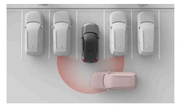
Your vehicle can detect a vehicle crossing behind you: for example, when reversing out of a parking spot. This allows it to warn you so that you can slow down or brake.
