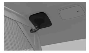
**3** Fasten the lower corners of the net to the outer tether points behind the seats.
