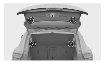
There are two attachment points on the parcel shelf itself and two on the trunk hatch. When the parcel shelf is attached, cords run between attachment points on the parcel shelf and the trunk hatch.
