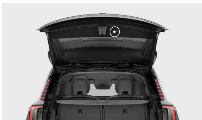
Location of the trunk closing button
