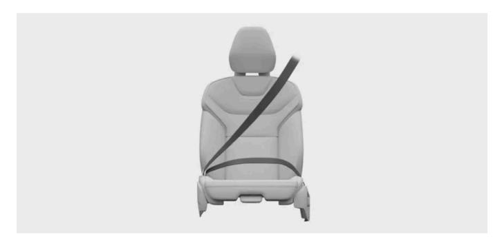
The seat belt locks itself to act as a safety restraint under certain conditions, such as sudden and forceful pulling of the belt, if the vehicle is driven aggressively and if the vehicle is on a steep incline.
