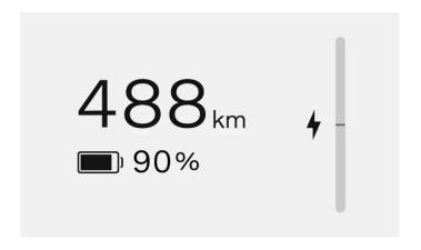
Your range is primarily related to your vehicle's battery level and your driving practices, but external conditions can also be a factor. The battery level and expected range are displayed in the instrument panel. The expected range is calculated based on your driving pattern, both current and historical.
