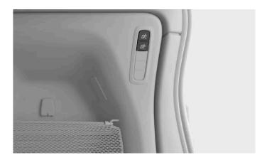
On the right-hand side in the trunk, there is a button panel. The top two buttons, one for each seat, can be used to fold and raise the third-row seats. This location can be useful if you need more room for stowing while using the trunk.
