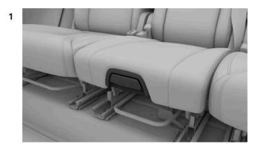
Pull the handle on the front of the center seat cushion to release the lock.
