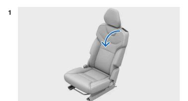
Pull the handle on the top of the outer seat backrest.
