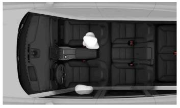
Left-side collision airbags for the front occupants. In a right-side collision, they deploy on the other side of each front seat (mirrored as compared with the depicted scenario).
