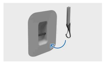
Fastening tether to top tether attachment point
