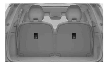
The top tether attachment point locations for the outer second-row seats and third-row seats are indicated by the top tether symbol.
