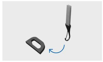
Fastening tether to lower tether attachment point
