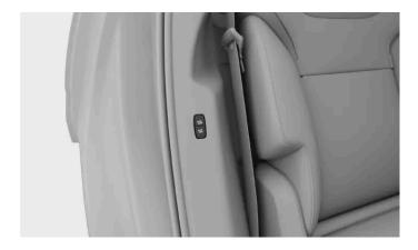
When a rear door is open, you can find the folding buttons in the door frame. There is one identical set of buttons on each side of the vehicle. These locations can be useful if you plan to fold both the second- and third-row seats .
