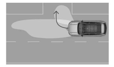
The cornering lights illuminate the area close to the vehicle to give you better visibility when turning.
