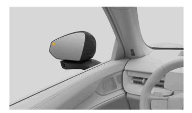
When a vehicle is detected in or approaching your blind spot, a light appears in the door mirror.
