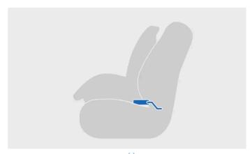
Child restraint installed using ISOFIX<sup>[1]</sup>
