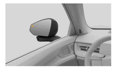
When the vehicle detects traffic that is about to pass close to the sides, a light appears in the door mirror. If you begin to open the door on the side of the detected traffic, the alert intensifies. An audible alert can occur along with the visual alerts, depending on how urgent the warning is.
