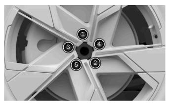
Tighten the wheel fasteners crosswise.
