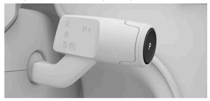
> The vehicle transitions to a parked state, which includes engaging the parking brake. The new state is indicated in the instrument panel.
