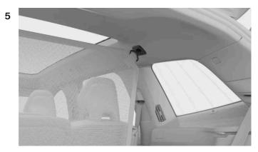
Insert each pin of the safety net into the sockets at the sides of the inner roof. Push the pins forward until they lock into place.
