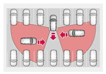
Examples of areas in which the function can help the driver detect obstacles while backing up.
