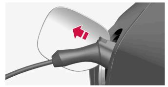
Press the release button on the charging cable's handle. The handle will be released/unlocked. Unplug the cable from the vehicle's charging socket and close the charger door.
