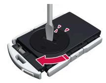
Put the battery cover back into place and turn it clockwise to the CLOSE position.
