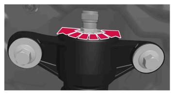
Turn the adjustment knob clockwise or counterclockwise to change the adjustment position.
