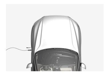
The hybrid battery is recharged using the charging cable. It can also be recharged during light braking and through engine braking in gear position B. The combustion engine can also help recharge the hybrid battery. The vehicle's start battery is charged when the hybrid battery is charged.
