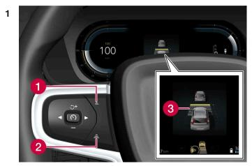
Controls for setting a time interval.
