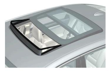
The panoramic roof is equipped with a wind blocker that folds up when the roof is open.
