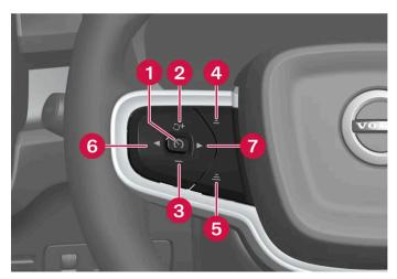
Buttons for speed-controlling functions
