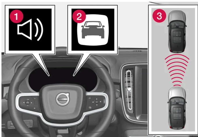
Collision warning audible signal and symbol
