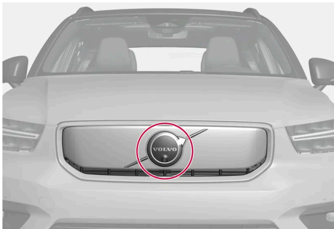
Location of the front radar sensor
