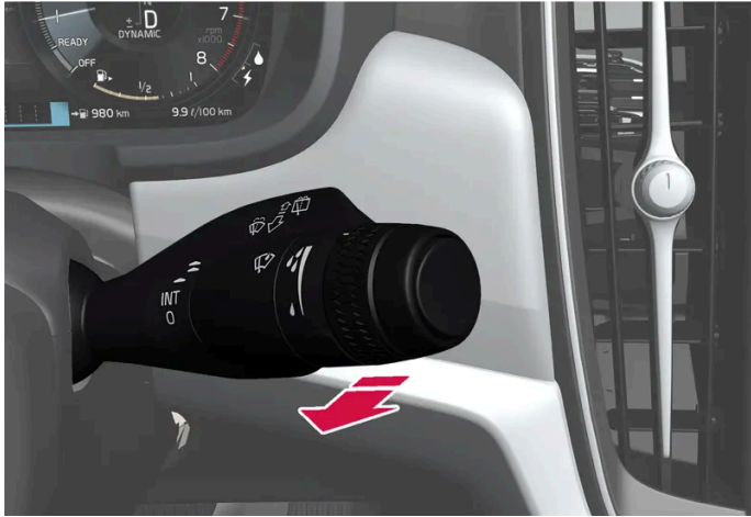
Washing function, right-hand steering wheel lever.
