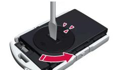
Turn the battery cover counterclockwise to the OPEN position. Use a screwdriver, coin or similar.
