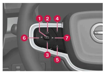
Buttons for speed-controlling functions
