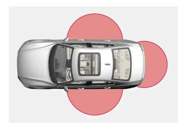
For keyless operation to be possible, the key must be within a distance of about 1 to 1.5 meters (3 to 5 feet) from the vehicle's doors or trunk lid.
