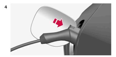
Remove the charging handle's protective cover and push the charging handle all the way into the vehicle's socket.
