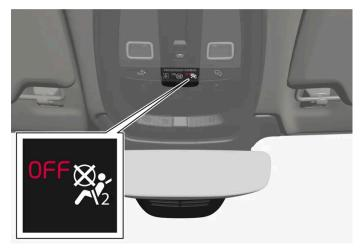
Occupant Weight Sensor (OWS) indicator light
