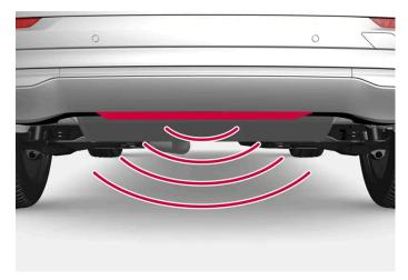
The sensor is located in the center under the bumper.
