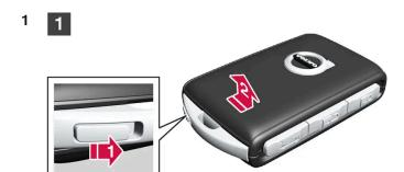
Move the catch next to the key ring bracket to the side and slide the front cover away from the bracket.
