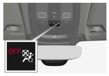
Occupant Weight Sensor (OWS) indicator light
