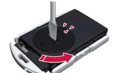
Turn the battery cover counterclockwise to the OPEN position. Use a screwdriver, coin or similar.
