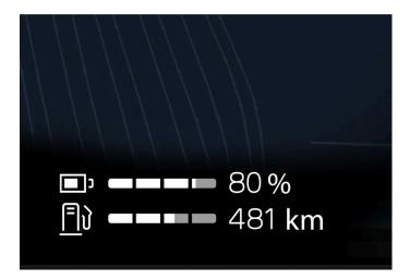
The battery gauge at the bottom of the instrument panel shows the charge level of the battery and the estimated driving distance until the battery is discharged.
