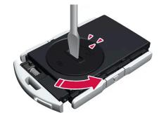
Turn the battery cover counterclockwise to the OPEN position. Use a screwdriver, coin or similar.
