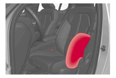
The near-side airbags are located in the front seats' outer backrest frames and help protect the driver and front-seat passenger.
