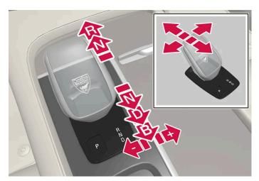
Gear selector and gear selector positions overview.
