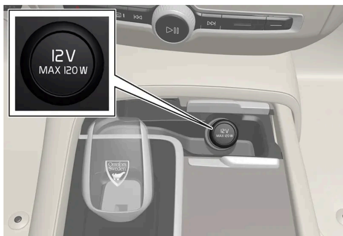
Front electrical outlet in the tunnel console for vehicles with wireless phone charger*.
