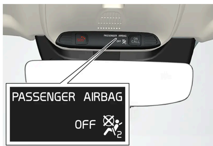
Occupant Weight Sensor (OWS) indicator light
