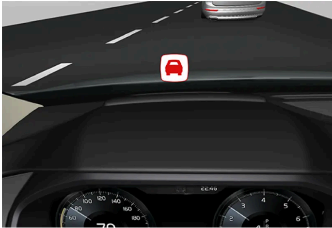
Collision warning symbol on the windshield
