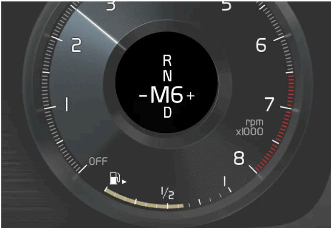
Overview of manual gear selector positions in instrument panel.
