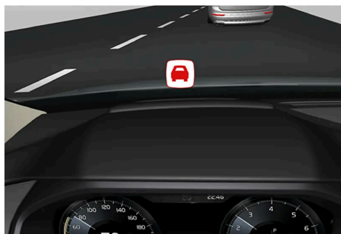
Collision warning symbol on the windshield
