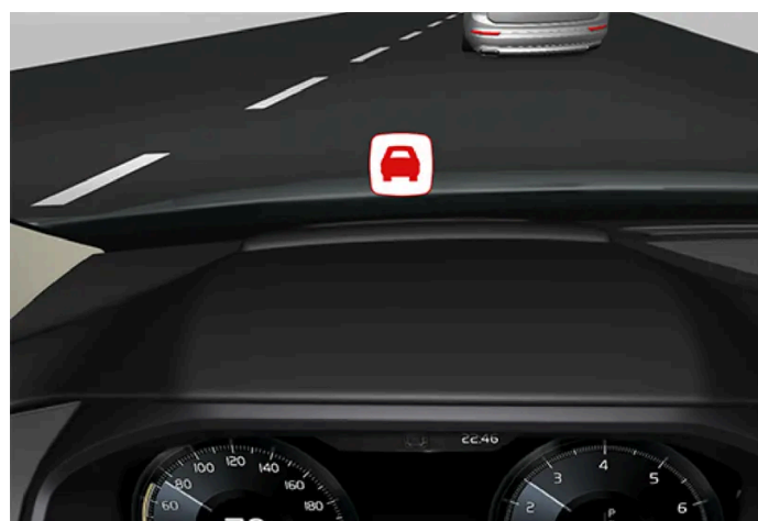
Collision warning symbol on the windshield
