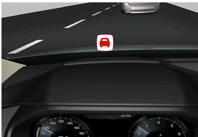
Collision warning symbol on the windshield
