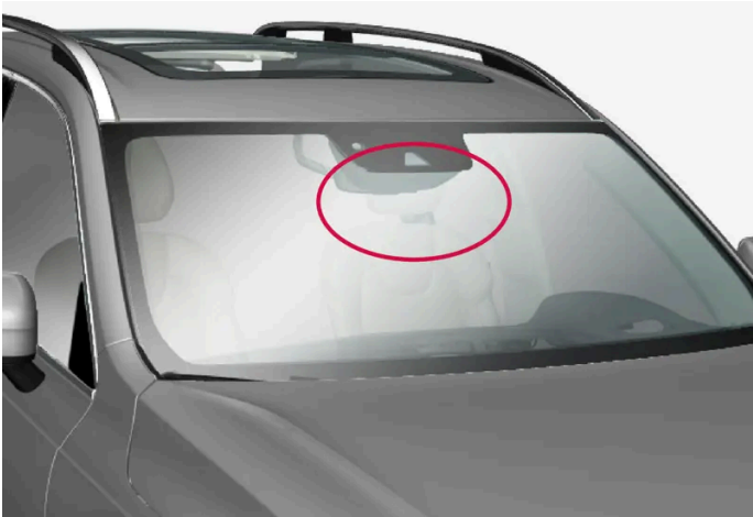
Location of the front radar sensor
