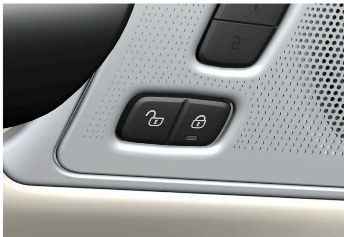
Lock buttons with indicator lights in front door.
