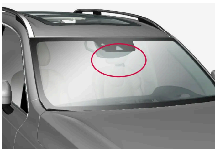
Location of front camera and radar sensor
