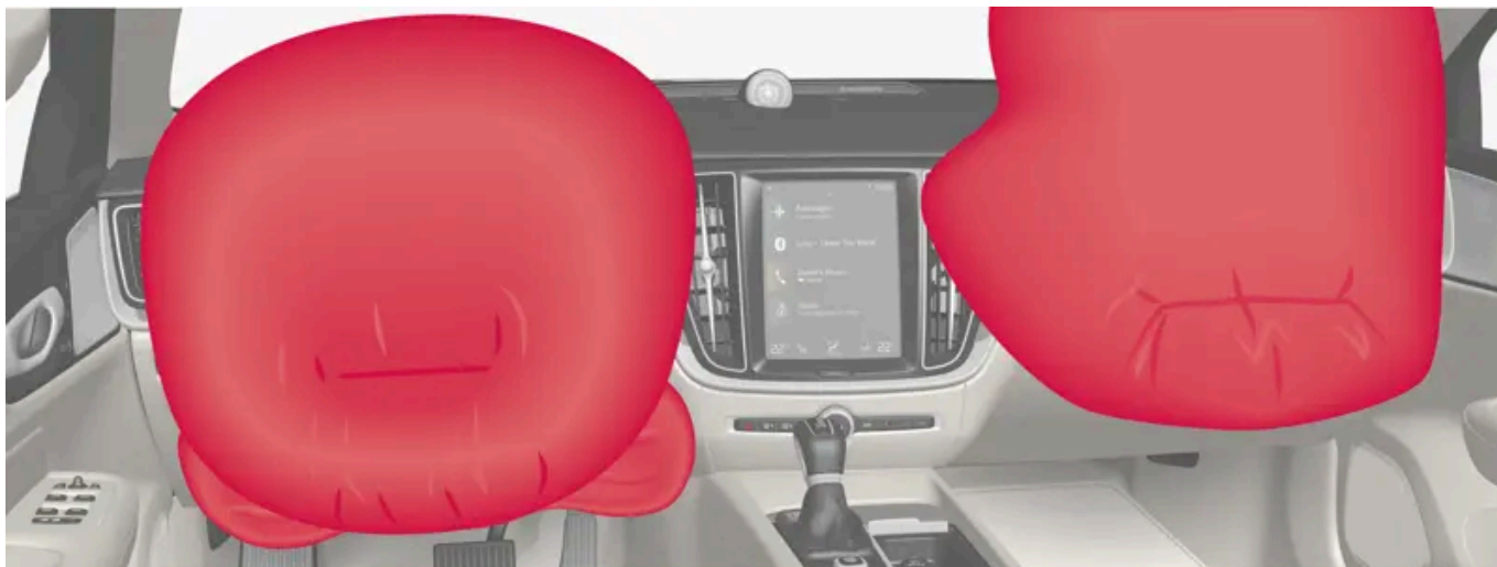
Driver/passenger side front airbags.
