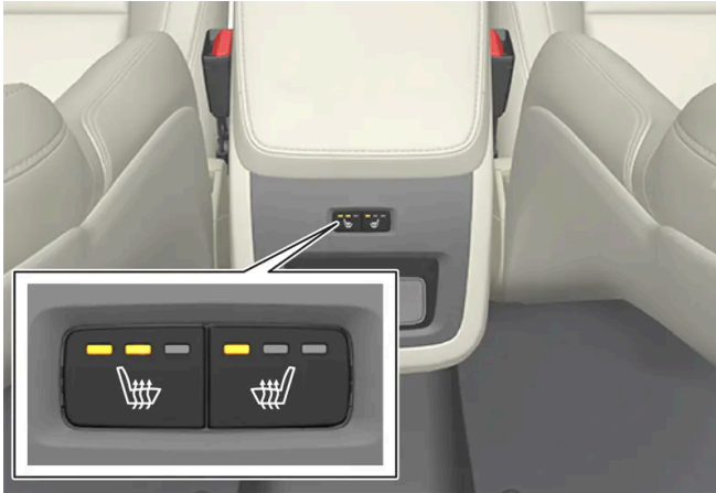
Buttons for seat heating on the rear side of the tunnel console.
