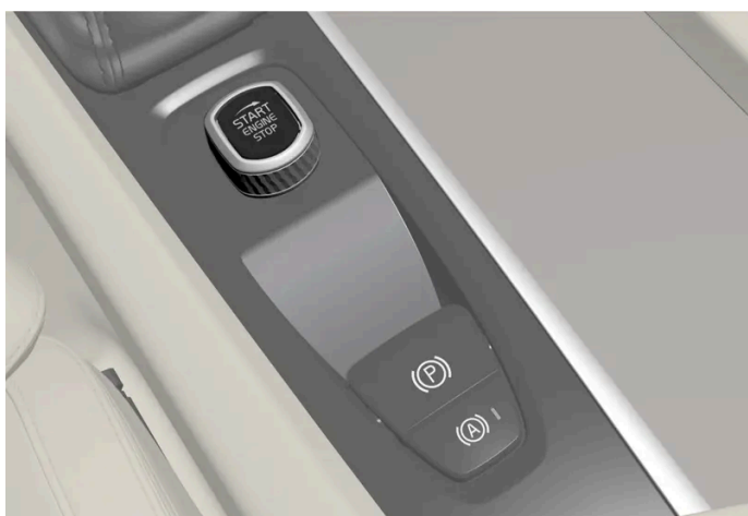
Start knob in the tunnel console.
