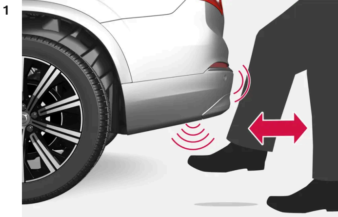
Kicking motion within the sensor's activation area.
