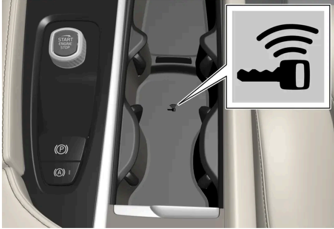
Location of the backup reader in the tunnel console.
