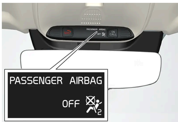
Occupant Weight Sensor (OWS) indicator light
