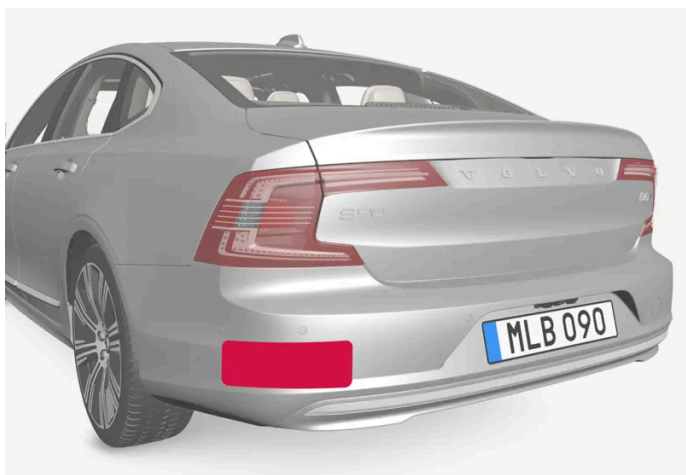
Location of rear radar sensors
