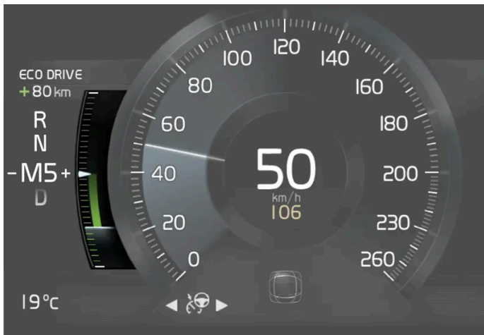
Eco gauge in 8" instrument panel.
