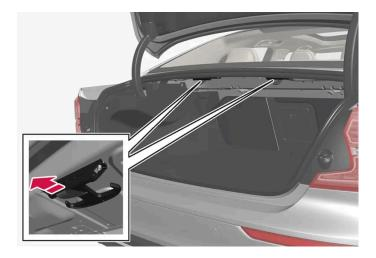
Fold down the hook from underneath the parcel shelf. Bags with handles of a suitable height can be hung from the hooks.
