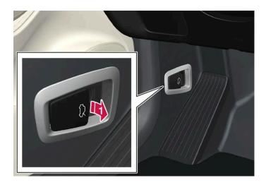
Pull the lever next to the pedals to release the hood from its fully closed position.
