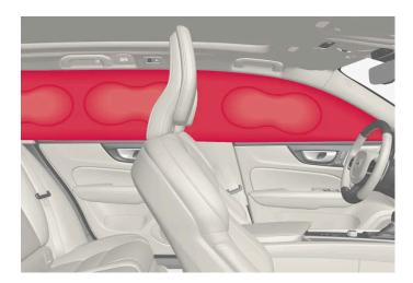
The inflatable curtains are installed along both sides of the inside of the roof and help protect occupants in the vehicle's outer seats. IC AIRBAG is embossed on the panels.
