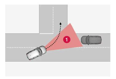
1 Sector in which the function can detect an oncoming vehicle in crossing traffic.
