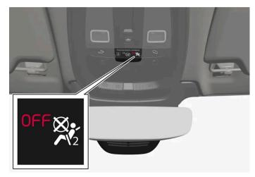
Occupant Weight Sensor (OWS) indicator light
