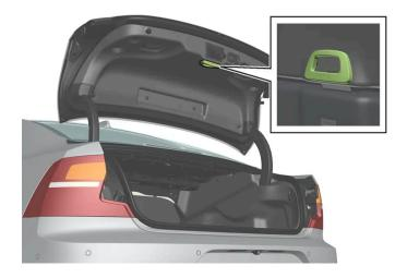
1 Pull the handle downward to release the trunk lid.
