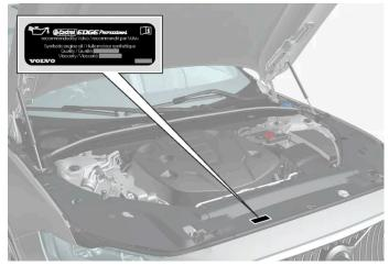
Location of warning decal for the engine compartment. The layout of the engine compartment may vary depending on model and engine variant.
