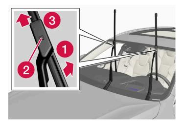
Raise the wiper arms to the service position. Service position is activated/deactivated via the center display when the vehicle is stationary and the windshield wipers are not on.
