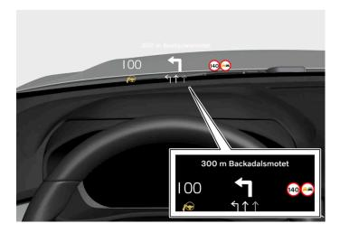
The head-up display projects information from the instrument panel onto the windshield in front of the driver. This information can only be seen from the driver's position.
