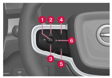
Buttons for speed-controlling functions
