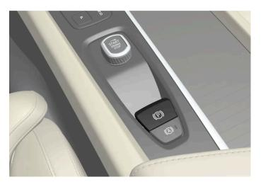
The parking brake controls are located in the tunnel console between the seats.
