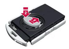
Insert a new battery with the positive side (+) facing upward. Do not touch the contact surfaces of the key battery. Place the edge of the battery under the two lower plastic catches.
