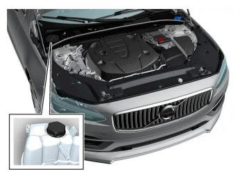
Coolant expansion tank, left-hand drive vehicle.
