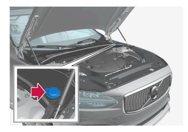
When there is approximately 1 liter (1 qt) of washer fluid remaining, the message **Refill washer fluid, level low** and the symbol will be displayed in the instrument panel.
