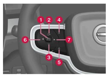
Buttons for speed-controlling functions
