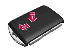
Put the back cover on in the reverse order it was removed. The back cover does not have a logo. Press the cover down until it clicks and then push it the last few millimeters back to its original position.
