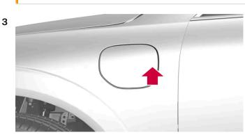
Press the rear edge of the charger door to open the charging socket<sup>[2]</sup>.
