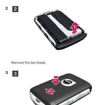
Put the front cover on in the reverse order it was removed. Press the cover down until it clicks and then push it the last few millimeters back to its original position.
