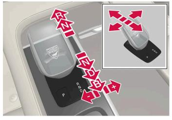
Gear selector and gear selector positions overview.
