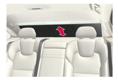
An electrically operated sun curtain is integrated in the rear window shelf.
