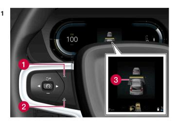
Controls for setting a time interval.
