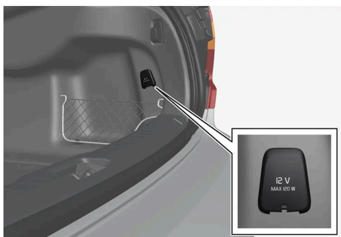
12 V outlet in trunk/cargo compartment*.
