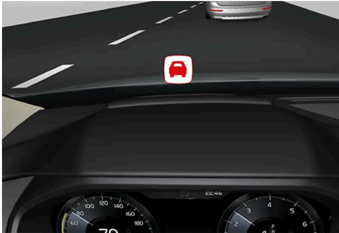
Collision warning symbol on the windshield
