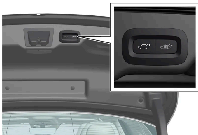
Location of button on underside of trunk lid.
