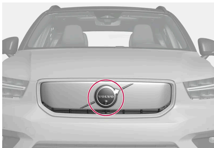
Location of the front radar sensor
