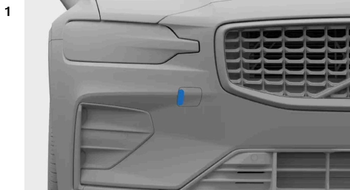
Front towing eye fastening cover
