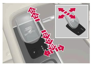
Gear selector and gear selector positions overview.
