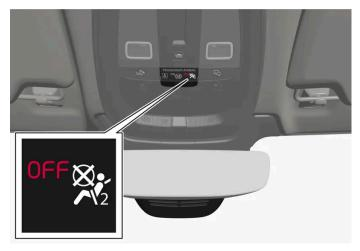
Occupant Weight Sensor (OWS) indicator light
