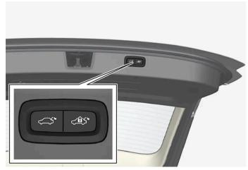
Location of button(s) on underside of tailgate.
