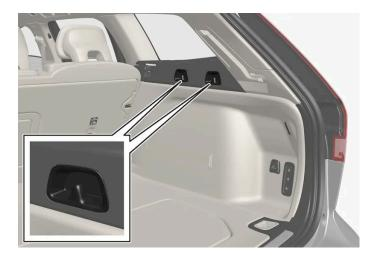
There are two grocery bag holders in the side panel on each side of the cargo compartment.
