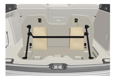
There are two grocery bag holders and an elastic band [1] in the hatch in the cargo compartment floor. The strap can be attached in four different positions.
