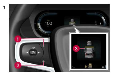
Controls for setting a time interval.
