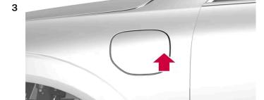
Press the rear edge of the charger door to open the charging  $socket^{[2]}$ .
