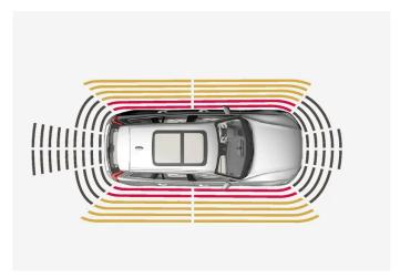
The warning signal pulsates rapidly when the obstacle is less than approx. 25 cm (0.8 foot) from the vehicle.
