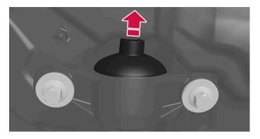
The rubber cap is located above the adjustment knob.
