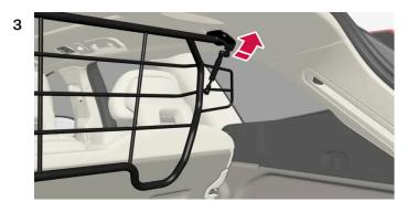
Position the grid's attachment points in the ceiling brackets.
