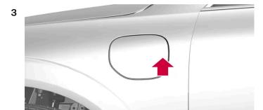
Press the rear edge of the charger door to open the charging  $socket^{[2]}$ .
