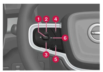
Buttons for speed-controlling functions
