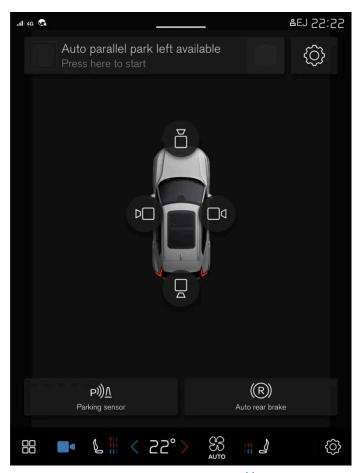
Camera view shows the Park Assist Cameras (PAC<sup>[1]</sup>), which display a 360° panoramic view as well as separate views for each of the four cameras: rear, front, left and right.
