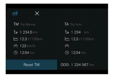
old – Information about trip odometer, odometer, etc.
