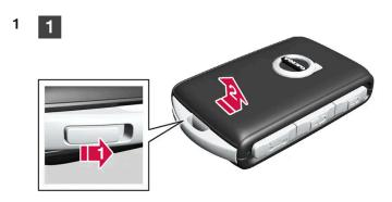
Move the catch next to the key ring bracket to the side and slide the front cover away from the bracket.
