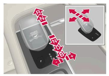
Gear selector and gear selector positions overview.
