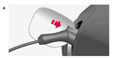
Remove the charging handle's protective cover and push the charging handle all the way into the vehicle's socket.
