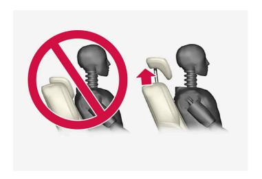
The center head restraint should be adjusted to suit the passenger's height. The entire back of the head should be covered if possible. Manually move the restraint up or down as needed.
