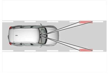
Driver Alert detects the vehicle's position in the traffic lane.
