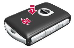
Turn the key and put the front cover back on in the same way as the back cover.
