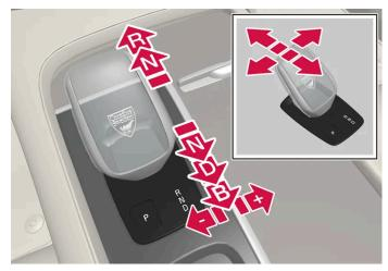
Gear selector and gear selector positions overview.
