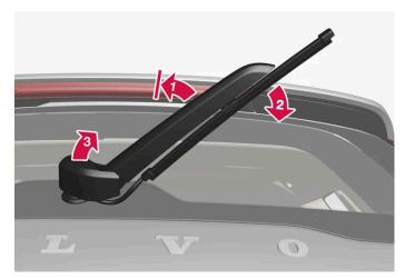
Lift the wiper arm from the window and pull the upper section of the blade down diagonally to the right.
