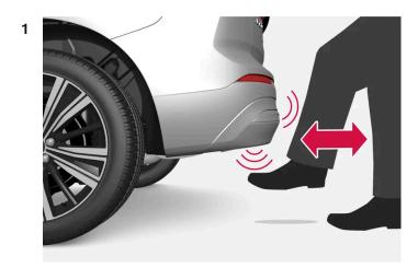
Make one forward kicking motion with your foot under the sensor area under the rear bumper. Then take a step back. Do not touch the bumper.
