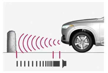
The warning signal has a continuous audible tone when the obstacle is less than approx. 30 cm (1 foot) from the vehicle.
