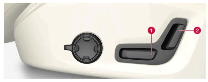
Move the passenger seat forward/rearward by moving the control forward/rearward.
