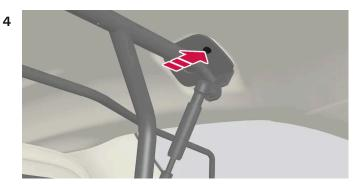
Screw the provided screw into place using the provided 6 mm Allen wrench. Repeat on the other side. Recommended torque: 20 Nm (15 lb-ft).
