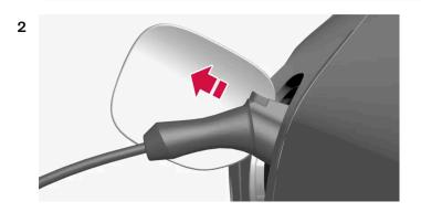
Press the release button on the charging cable's handle. The handle will be released/unlocked. Unplug the cable from the vehicle's charging socket and close the charger door.
