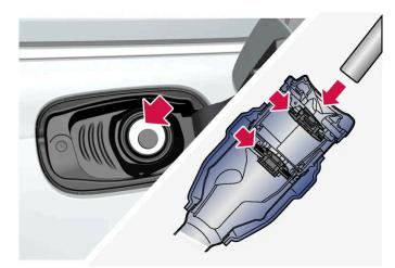
It is important to insert the pump's nozzle past both of the two flaps in the fuel filler pipe before beginning fueling.
