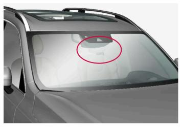
Location of front camera and radar sensor
