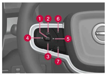
Buttons for speed-controlling functions
