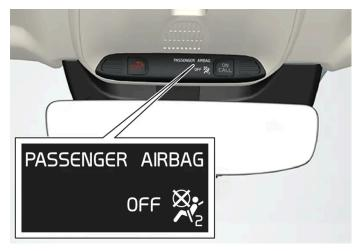
Occupant Weight Sensor (OWS) indicator light
