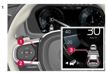
Controls for setting a time interval.
