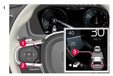
Controls for setting a time interval.
