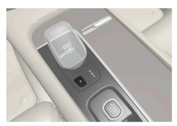
Overview of gear selector and gear position  $\ensuremath{\mathsf{P}}$  for the small gear selector.
