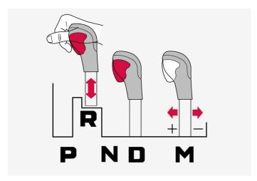
Shiftlock for vehicles with large gear selectors.
