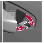
Pull the front left-hand door handle to its end position to access the lock cylinder.
