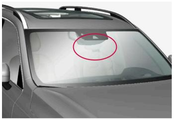
Location of front camera and radar sensor
