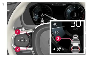
Controls for setting a time interval.
