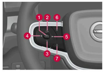
Buttons for speed-controlling functions
