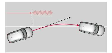
Lane Keeping Aid alerts the driver using vibrations in the steering wheel.
