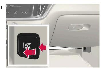
Insert a personal SIM card in the holder in the passenger-side footwell. Note that the vehicle's card reader requires **mini SIM** cards.
