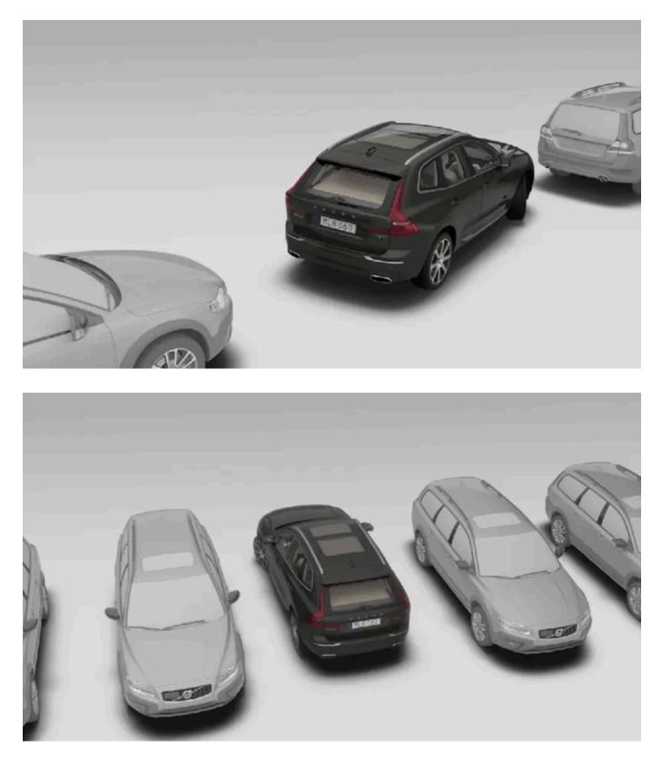
The function first checks whether there is sufficient space and then helps the driver steer the vehicle into the space.
