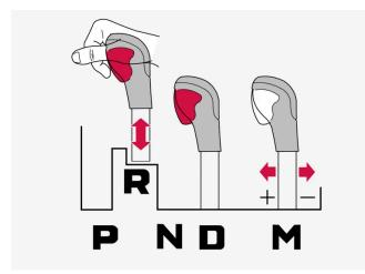
Shiftlock for vehicles with large gear selectors.
