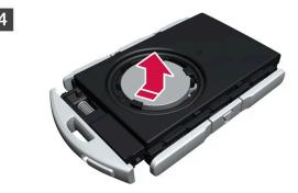
The battery's positive side (+) faces upward. Remove the battery by pressing its edge and then lifting it out.
