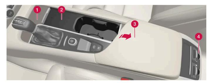
1 Storage compartment with cover\* and 12 V socket<sup>[1]</sup>. The cover can be opened/closed by pressing the handle.
