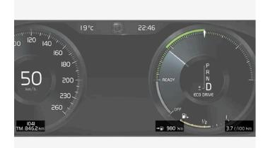
Example of trip computer information in a 12-inch instrument panel\*. The illustration is generic - details may vary according to vehicle model.
