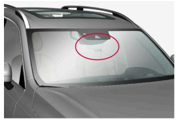
Location of front camera and radar sensor
