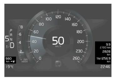
Example of trip computer information in an 8-inch instrument panel. The illustration is generic - details may vary according to vehicle model.
