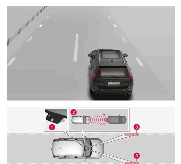
The camera/radar sensor monitors the distance to the vehicle ahead and detects lane markings.
