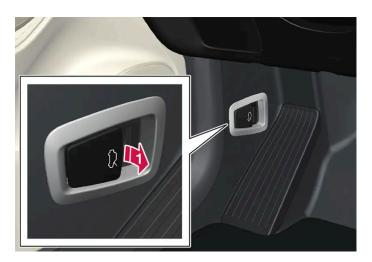
Pull the lever to the side of the pedals to release the hood from its fully closed position.
