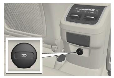
USB ports (type C) on rear of tunnel console for charging devices such as phones and tablets<sup>[1]</sup>.
