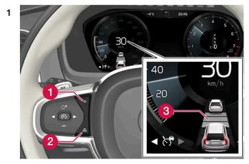
Controls for setting a time interval.
