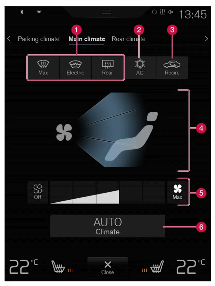
**1** Max, Rear – Controls for defrosting windows and door mirrors.
