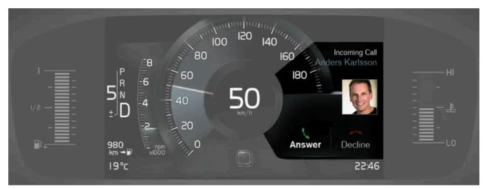
Example of message in an 8-inch instrument panel. The illustration is generic - details may vary according to vehicle model.
