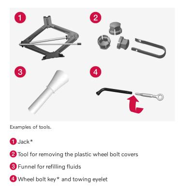
If the vehicle is equipped with a spare tire \* <sup>[1]</sup>, a jack and wheel bolt key are provided instead of the tire sealing system.
