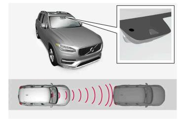
The camera/radar sensor measures the distance to the vehicle ahead.
