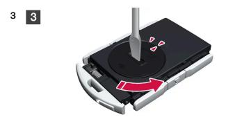
Turn the battery cover counterclockwise to the OPEN position. Use a screwdriver, coin or similar. Remove the battery cover. If it is difficult to remove, use a narrow object to carefully pry it up.
