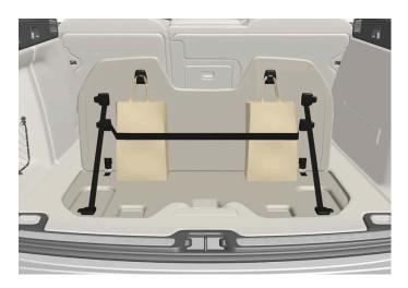
There are two grocery bag holders and an elastic band<sup>[1]</sup> in the hatch in the cargo compartment floor. The strap can be attached in four different positions.
