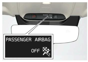
Occupant Weight Sensor (OWS) indicator light
