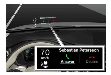
The head-up display projects warnings and information related to speed, cruise control functions, navigation, etc. onto the windshield in the driver's field of vision. Traffic information and incoming phone calls can also be shown on the head-up display.
