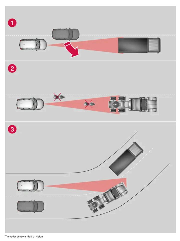
1 The radar sensor's detection of vehicles very close to your vehicle may be delayed in certain situations, e.g. if a vehicle pulls in between your vehicle and the vehicle directly ahead.
