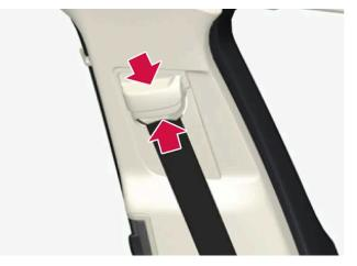
Press the button on the seat belt holder and move the belt up or down.
