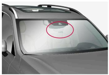
Location of front camera and radar sensor
