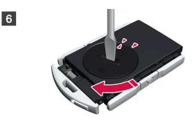
Put the battery cover back into place and turn it clockwise to the CLOSE position.
