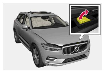
2 Swipe your hand from left to right under the hood, grasp the handle and move it up and to the side to release the catch and lift the hood.
