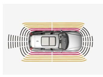
The warning signal pulsates rapidly when the obstacle is less than approx. 25 cm (0.8 foot) from the vehicle.
