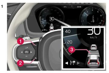
Controls for setting a time interval.
