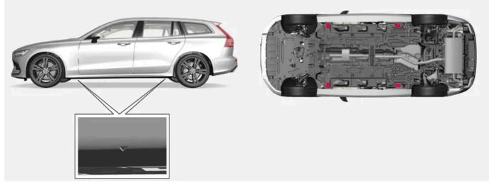
Arrows along the lower edges of the sides of the vehicle indicate the location of the jack attachment points/lifting points (shown in red).
