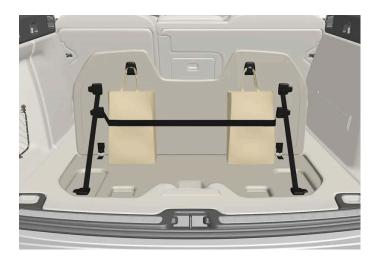
There are two grocery bag holders and an elastic band<sup>[1]</sup> in the hatch in the cargo compartment floor. The strap can be attached in four different positions.
