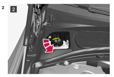
Unscrew the expansion tank cap and fill coolant as needed. The level should be between the MIN and MAX marks on the expansion tank.
