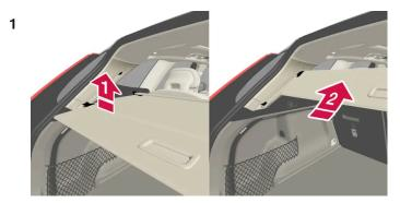
Press the handle section of the cargo compartment slightly upward.
