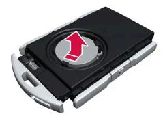
The battery's positive side (+) faces upward. Remove the battery by pressing its edge and then lifting it out.
