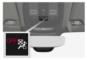
Occupant Weight Sensor (OWS) indicator light
