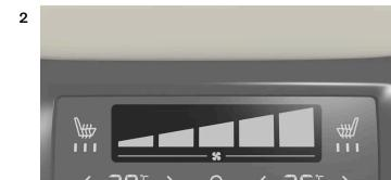
Blower controls on the rear climate panel of the tunnel console.
