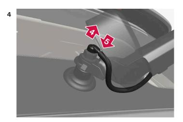
Remove the washer hose from the attachment.
