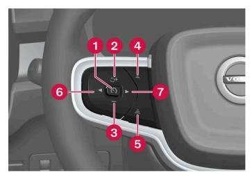
Buttons for speed-controlling functions
