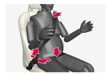
The seat belt should fit closely against the shoulder, with the diagonal section between the breasts and to the side of the stomach.
