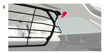
Position the grid's attachment points in the ceiling consoles.
