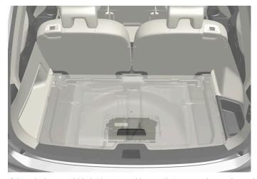
If the vehicle is a mild hybrid, it instead has a 48 V support battery located under the cargo compartment. The box over the 48 V support battery may only be handled by an authorized workshop.
