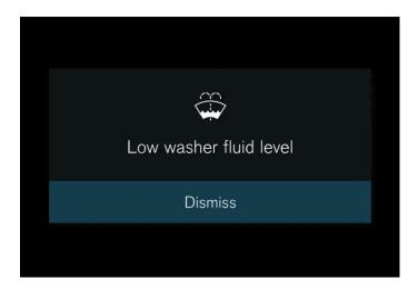
The messages are shown in the center of the instrument panel. The layout may vary and include graphics, symbols or buttons to e.g. acknowledge the message or accept a request.
