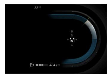
With position M, it is possible to shift gears manually. Engine braking will occur when the accelerator pedal is released.
