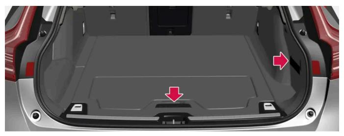
Cargo compartment with elastic band and storage space under the cargo compartment floor.
