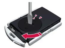
Put the battery cover back into place and turn it clockwise to the CLOSE position.
