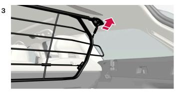
Position the grid's attachment points in the ceiling consoles.
