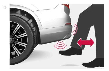
Make one forward kicking motion with your foot under the sensor area under the rear bumper. Then take a step back. Do not touch the bumper.
