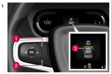
Controls for setting a time interval.
