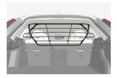
For safety reasons, the steel grid must always be installed and secured correctly.
