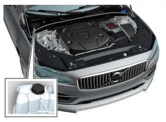
Coolant expansion tank, left-hand drive vehicle.
