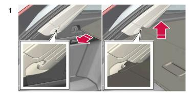
Grasp the handle and pull the cover out and above the side panels in the cargo compartment. Pull the cover to its end position.
