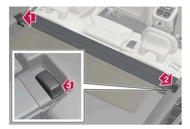
Press the end piece on one side of the cover into the retaining bracket in the side panel of the cargo compartment.
