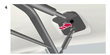
Screw the provided screw into place using the provided 6 mm Allen wrench. Repeat on the other side. Recommended torque: 20 Nm (15 ft-lb).
