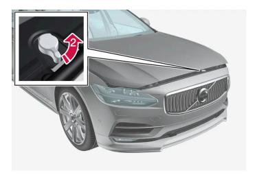
Turn the handle under the hood counterclockwise to release the catch and lift the hood.
