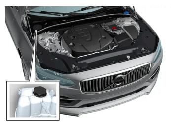
Coolant expansion tank, left-hand drive vehicle.
