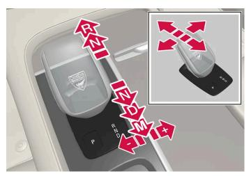
Gear selector and gear selector positions overview.
