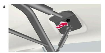
Screw the provided screw into place using the provided 6 mm Allen wrench. Repeat on the other side. Recommended torque: 20 Nm (15 lb-ft).
