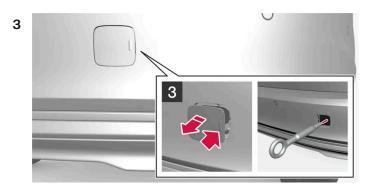
Rear: Remove the cover by pressing on the mark with a finger while folding out the opposite side/corner.
