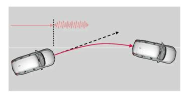
Lane Keeping Aid alerts the driver using vibrations in the steering wheel.
