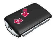
Put the back cover on in the reverse order it was removed. The back cover does not have a logo. Press the cover down until it clicks and then push it the last few millimeters back to its original position.
