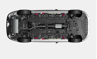
The vehicle has outer lifting points for smaller lifts, and inner lifting points for larger lifts with a garage hoist, lifting arms, etc.
