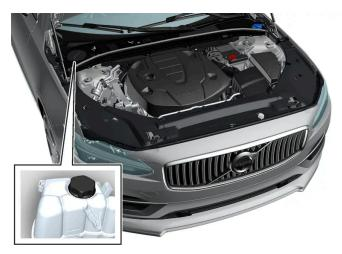
Coolant expansion tank, left-hand drive vehicle.
