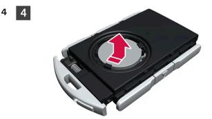
The battery's positive side (+) faces upward. Remove the battery by pressing its edge and then lifting it out.
