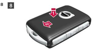
Turn the key and put the front cover back on in the same way as the back cover.
