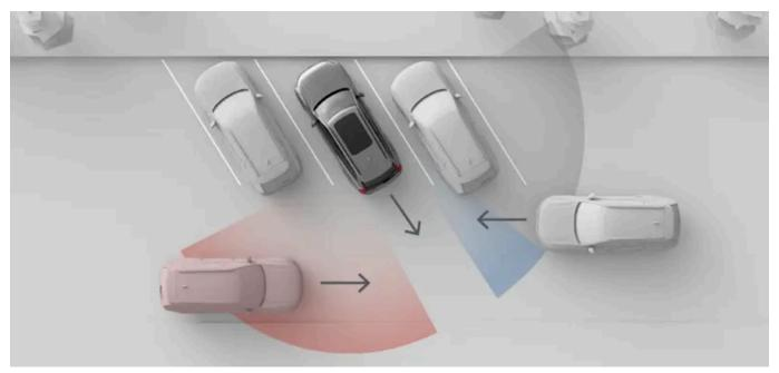
The situation in this image illustrates how surrounding objects such as parked vehicles can limit the vehicle's ability to detect other vehicles and traffic situations. In a situation without obstacles, the effective detection zones are the same on both sides.
