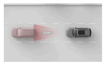
If the motorcycle and the larger vehicle are close to each other, they may appear to overlap to the detection systems, making detection of the motorcycle less accurate.
