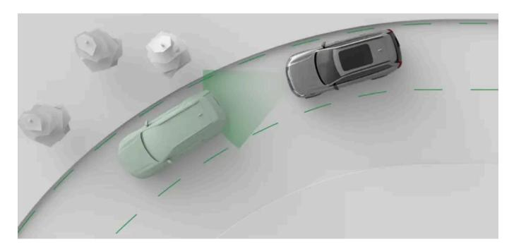
Pilot Assist actively guides your driving in a number of ways. When driving with Pilot Assist, you select the target speed. The vehicle then manages acceleration and braking to meet that target while also adapting to surrounding traffic.
