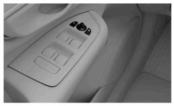
Controls for adjusting the door mirrors
