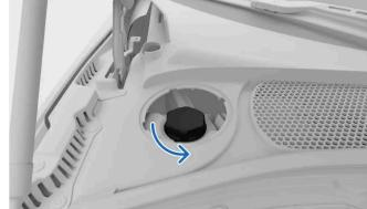
Unscrew the coolant reservoir cap.
