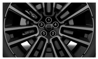
Tighten the wheel fasteners crosswise.
