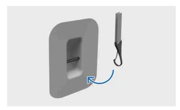
Fastening tether to top tether attachment point
