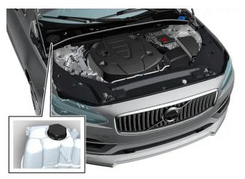
Coolant expansion tank, left-hand drive vehicle.
