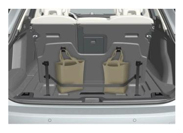
There are two grocery bag holders and an elastic band<sup>[1]</sup> in the hatch in the cargo compartment floor. The strap can be attached in four different positions.
