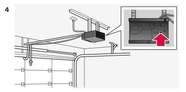
Locate the "training" button<sup>[2]</sup> on the receiver for the e.g. garage door opener. It is usually located near the antenna bracket on the receiver.
