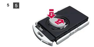
Insert a new battery with the positive side (+) facing upward. Do not touch the contact surfaces of the key battery.
