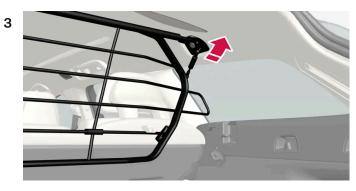
Position the grid's attachment points in the ceiling brackets.
