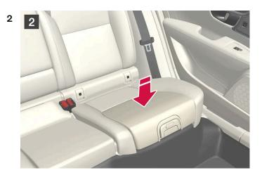
Press down on the center of the booster cushion to lock it into position.
