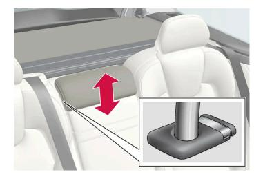
To lower the restraint, push and hold the button (see illustration) while carefully lowering the head restraint.
