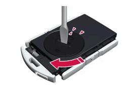
Put the battery cover back into place and turn it clockwise to the CLOSE position.
