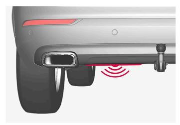
The sensor is located to the left of center under the rear bumper.
