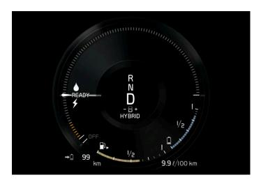
The vehicle has been started, but is stationary and no power is being requested.
