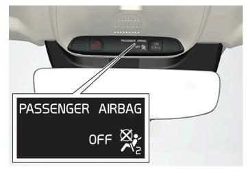
Occupant Weight Sensor (OWS) indicator light
