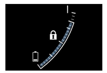
The firsymbol in the hybrid battery gauge indicates that the Hold function is activated. The first symbol indicates that the Charge function is activated.
