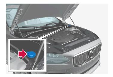
Fill washer fluid into the reservoir with the blue cover. The reservoir is used for the windshield washer, tailgate window washer and headlight washer\*.
