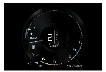
Indicator in the instrument panel during energy recovery.
