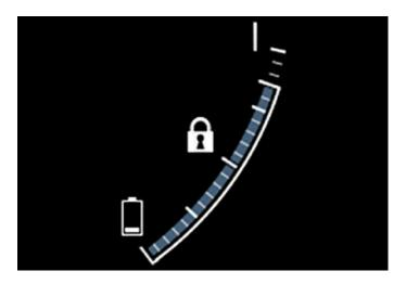
The first symbol in the hybrid battery gauge indicates that the Hold function is activated. The first symbol indicates that the Charge function is activated.
