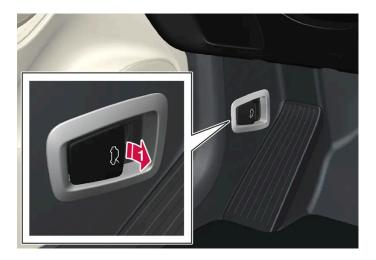
Pull the handle to the left of the brake pedal to release the hood from its fully closed position.
