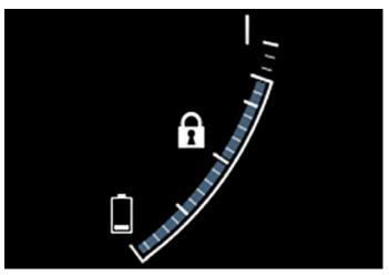
The fi symbol is displayed in the hybrid battery gauge when Hold is activated.
