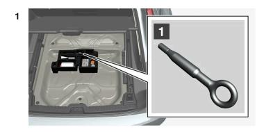
Take out the towing eyelet, which is stored in a foam block under the floor in the cargo compartment [1].
