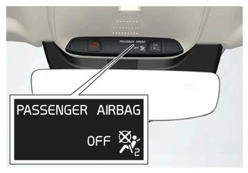
Occupant Weight Sensor (OWS) indicator light
