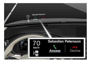
The head-up display projects warnings and information related to speed, cruise control functions, navigation, etc. onto the windshield in the driver's field of vision. Traffic information and incoming phone calls can also be shown on the head-up display.
