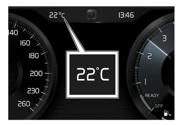
If the vehicle has been stationary, the sensor reading may be higher than the actual temperature.
