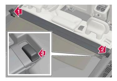
Press the end piece on one side of the cover into the retaining bracket in the side panel of the cargo compartment.
