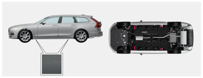
The triangles in the plastic covering indicate where the jack attachment points/lifting points (red areas) are located.
