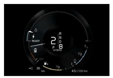
Indicator in the instrument panel during energy recovery.
