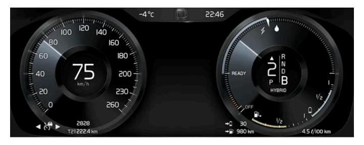
The instrument panel displays information such as speed, incoming phone calls or the track currently playing. It is controlled using the steering wheel keypads.
