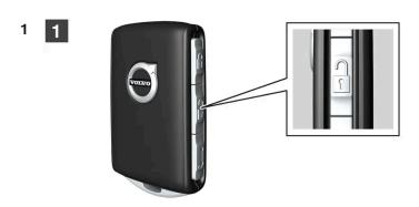
1 Unlock the vehicle with the remote key. Charging will stop.
