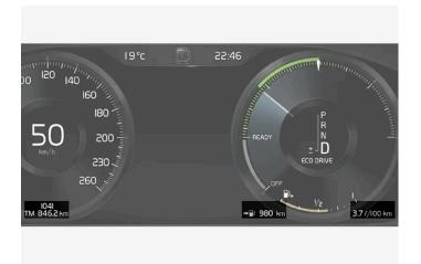
Example of trip computer information in the instrument panel. The illustration is generic - details may vary according to vehicle model.
