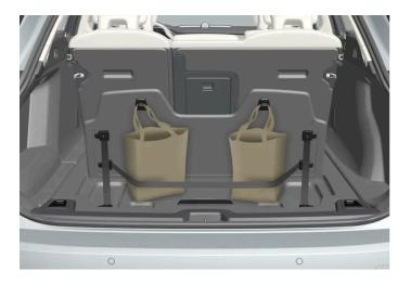
There are two grocery bag holders and an elastic band [1] in the hatch in the cargo compartment floor. The strap can be attached in four different positions.
