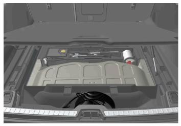
The charging cable is stored in a storage compartment under the cargo compartment floor.
