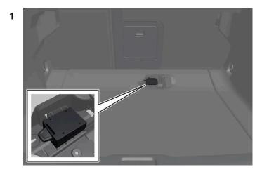
Insert a personal SIM card in the holder under the floor of the cargo compartment.
