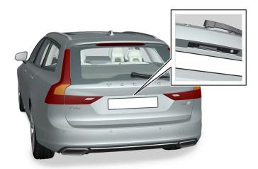
The rubberized button on the tailgate can only be used for unlocking.
