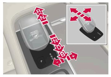
Gear selector and gear selector positions overview.
