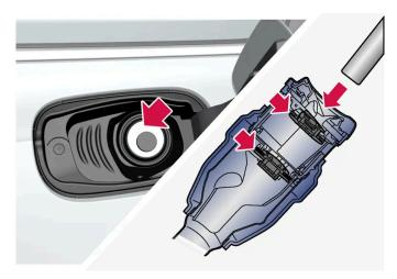
It is important to insert the pump's nozzle past both of the two flaps in the fuel filler pipe before beginning fueling.
