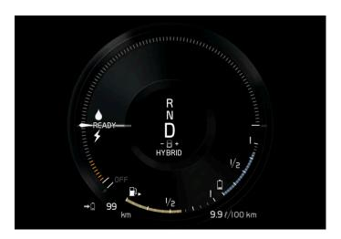
The hybrid gauge shows the ratio between the electric motor's current power consumption and the remaining available power. This information is shown in various ways.
