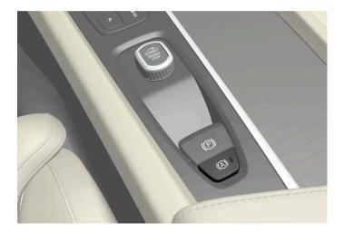
1 Press the button in the tunnel console to activate or deactivate the function.
