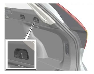
There are two grocery bag holders in the side panel on each side of the cargo compartment.
