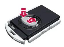
Insert a new battery with the positive side (+) facing upward. Do not touch the contact surfaces of the key battery.
