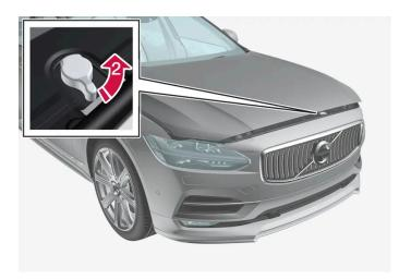
2 Turn the handle under the hood counterclockwise to release the catch and lift the hood.
