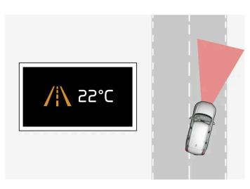
Indicates that the Lane Keeping Aid system is alerting the driver and/or attempting to steer the vehicle back into the lane.
