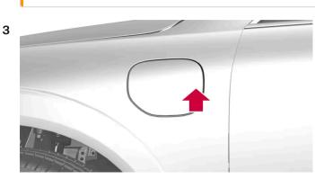
Press the rear edge of the charger door to open the charging socket<sup>[2]</sup>.
