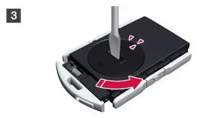
Turn the battery cover counterclockwise to the OPEN position. Use a screwdriver, coin or similar.
