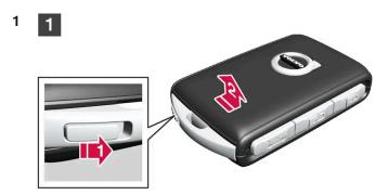
Move the catch next to the key ring bracket to the side and slide the front cover away from the bracket.
