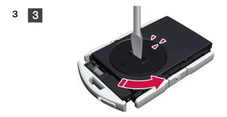
Turn the battery cover counterclockwise to the OPEN position. Use a screwdriver, coin or similar. Remove the battery cover. If it is difficult to remove, use a narrow object to carefully pry it up.
