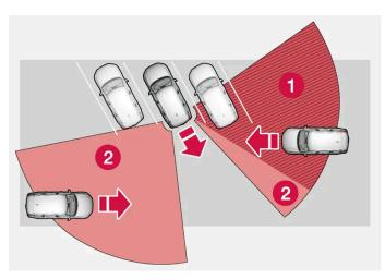
In a diagonal parking space, the sensors may be completely blocked on one side of your vehicle.
