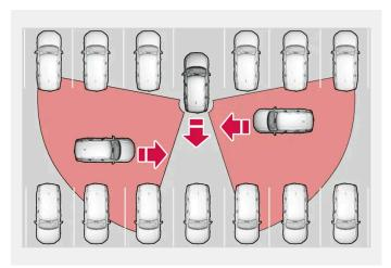
Examples of areas in which the function can help the driver detect obstacles while backing up.
