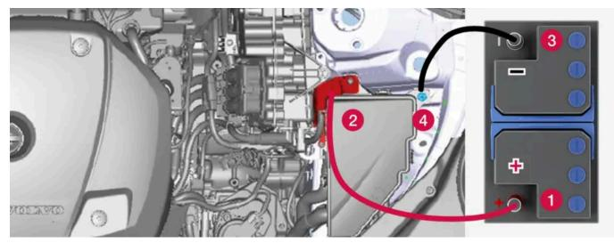
Jumper cable charging points. Engine compartment appearance may vary depending on vehicle model and equipment level.
