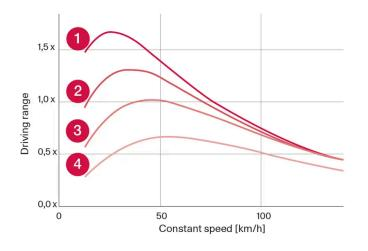
1 20 °C (68 °F) ambient temperature and passenger compartment climate control off.
