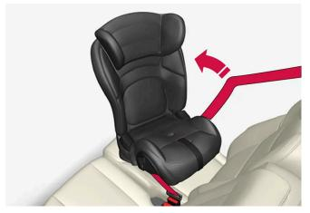
Pull out the shoulder section of the seat belt.
