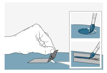
If the damage has not reached all the way down to the metal, then touch-up paint can be applied immediately after the surface has been cleaned.
