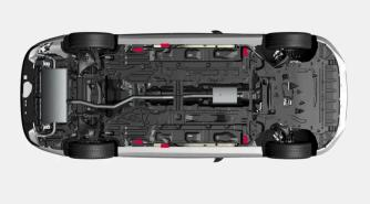
The vehicle has outer lifting points for smaller lifts, and inner lifting points for larger lifts with a garage hoist, lifting arms, etc.
