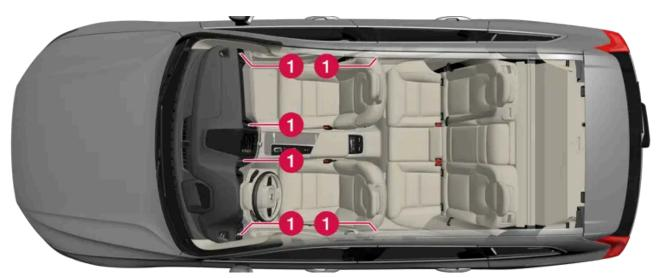
Location of adjustable air vents in the passenger compartment.
