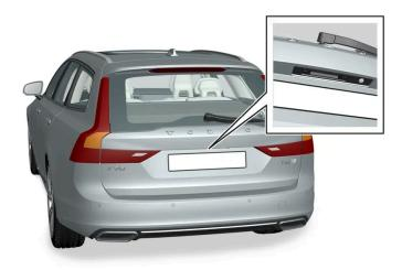
The tailgate is held closed by an electronic locking mechanism.
