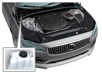
Coolant expansion tank, left-hand drive vehicle
