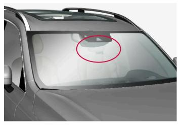
Location of front camera and radar sensor
