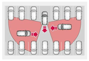
Examples of areas in which Cross Traffic Alert can help the driver detect obstacles while backing up.
