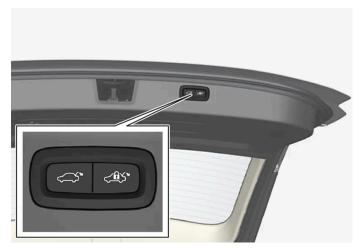
Location of button(s) on underside of tailgate.
