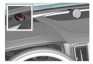
The locks and alarm indicator will display the status of the locking system:
