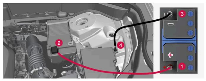
Jumper cable connecting points. Engine compartment appearance may vary depending on vehicle model and equipment level.
