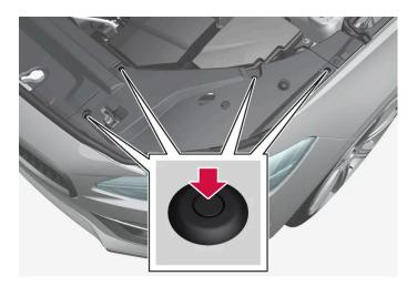
Release the pins in the plastic cover's four clips by pressing them down with a screwdriver or similar object and remove the covering.
