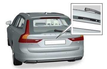
The rubberized button on the tailgate can only be used for unlocking.
