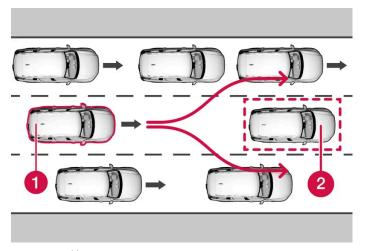
Your vehicle (1) cannot detect any potential escape routes for veering away from the vehicle ahead (2) and may therefore apply the brakes at an earlier stage.
