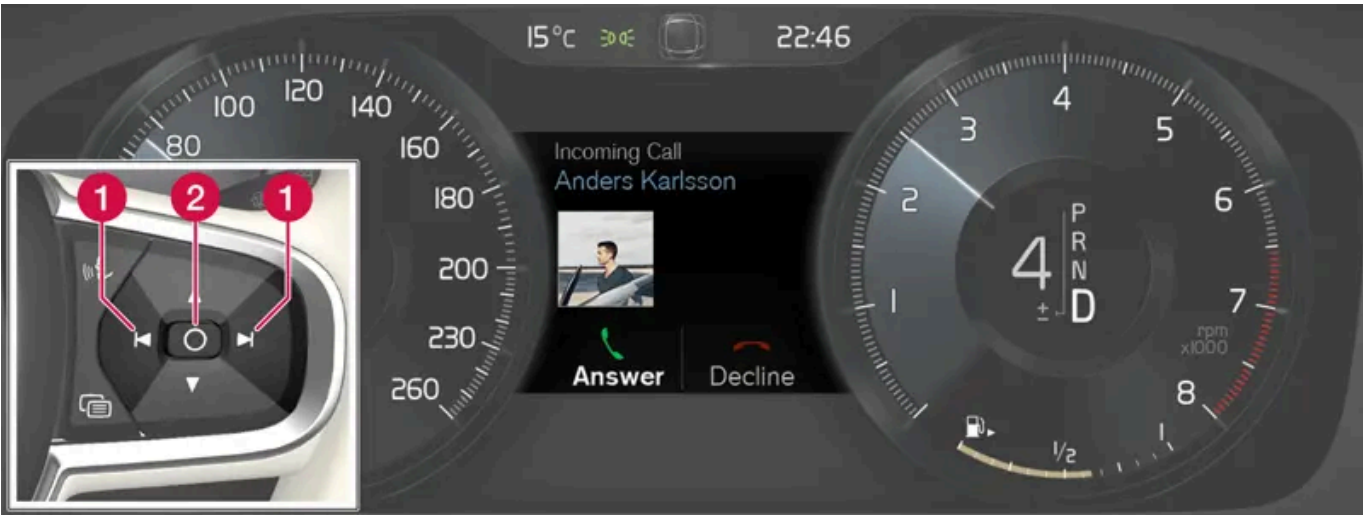
Examples of messages in the instrument panel [1] and the right-side steering wheel keypad. The illustration is generic - details may vary according to vehicle model.
