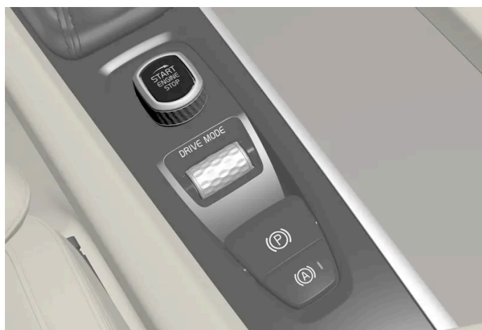
Start knob in the tunnel console.
