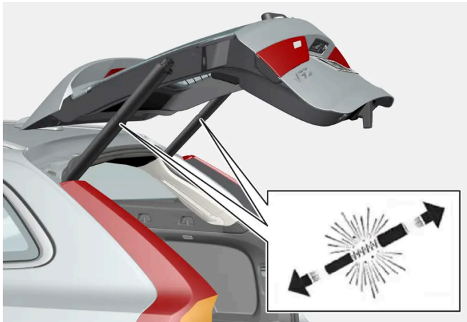
Preloaded springs for the power tailgate.
