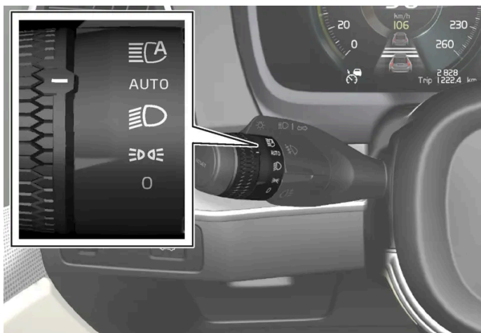
Lighting ring position.
