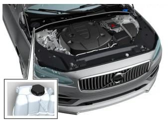
Coolant expansion tank, left-hand drive vehicle.
