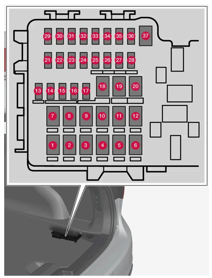
The fuse box is located behind the panel on the right-hand side.
