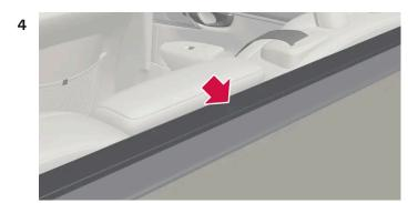
Fold out the cover's front flap to eliminate the gap between the cover and the rear seat backrest.
