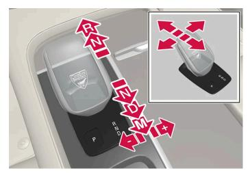
Gear selector and gear selector positions overview.
