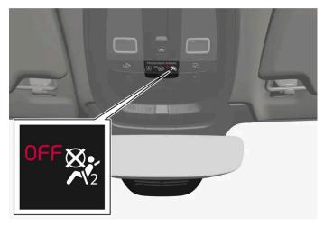
Occupant Weight Sensor (OWS) indicator light
