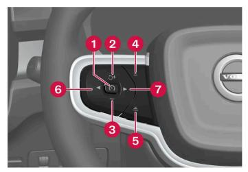
Buttons for speed-controlling functions
