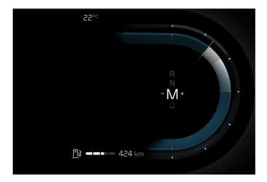
With position M, it is possible to shift gears manually. Engine braking will occur when the accelerator pedal is released.
