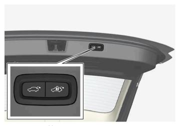
Location of button(s) on underside of tailgate.
