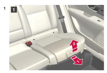
Pull the handle forward and upward to release the booster cushion.
