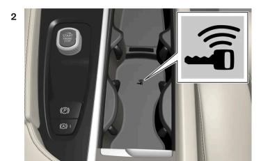
Place the key on the key symbol in the backup reader in the tunnel console's cup holder.
