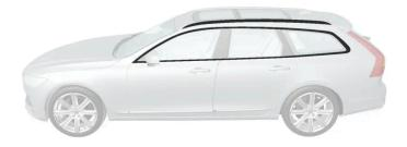
Components that should be washed with a cleaning product with a pH value between 3.5 and 11.5.
