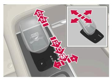
Gear selector and gear selector positions overview.
