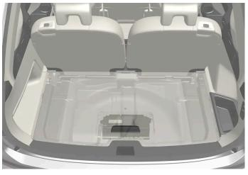
Mild hybrid vehicles have a 48 V support battery located under the cargo compartment. The battery and the box around it may only be handled by authorized workshop personnel.
