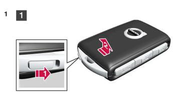
Move the catch next to the key ring bracket to the side and slide the front cover away from the bracket.
