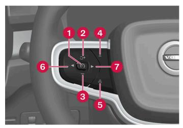
Buttons for speed-controlling functions
