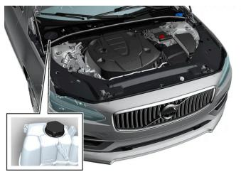
Coolant expansion tank, left-hand drive vehicle.
