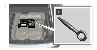
Take out the towing eyelet, which is stored in a foam block under the floor in the cargo compartment.
