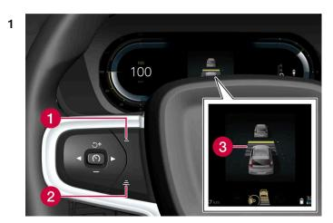
Controls for setting a time interval.
