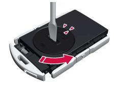
Turn the battery cover counterclockwise to the OPEN position. Use a screwdriver, coin or similar.
