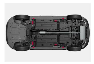
The vehicle has outer lifting points for smaller lifts, and inner lifting points for larger lifts with a garage hoist, lifting arms, etc.
