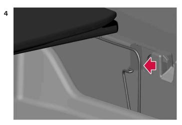
While continuing to hold the cargo compartment floor up, press the locking clip on the other side, as shown by the arrow.
