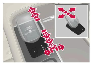
Gear selector and gear selector positions overview.
