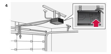
Locate the "training" button [2] on the receiver for the e.g. garage door opener. It is usually located near the antenna bracket on the receiver.
