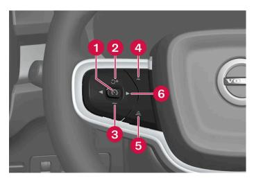
Buttons for speed-controlling functions
