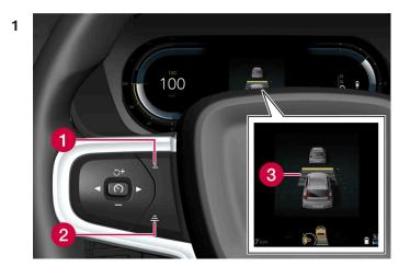
Controls for setting a time interval.
