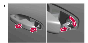
Pull the handle on the left-side front door to its end position.
