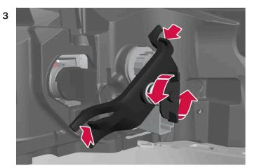
Unscrew the spring screw by turning counterclockwise, press the clips into the sides and remove the support bridge. It is simplest to leave one screw in place in the support bridge.
