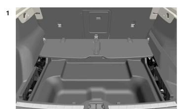
Fold the cargo compartment floor forward to position the parcel shelf with its top facing down and its rear part facing forward.
