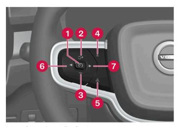
Buttons for speed-controlling functions
