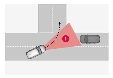
1 Sector in which the function can detect an oncoming vehicle in crossing traffic.
