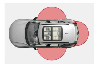
For keyless operation to be possible, the key must be within a distance of about 1 to 1.5 meters (3 to 5 feet) from the vehicle's doors or tailgate.
