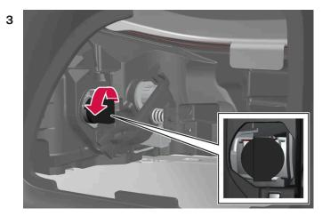
Remove the black bulb holder by turning it counterclockwise and pulling it out.
