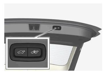
Location of button(s) on underside of tailgate.
