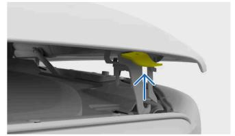
Locate the second lever on the underside of the hood and push it upward.
