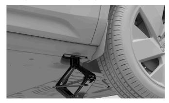
8 Raise the vehicle to an appropriate height. Do not raise it higher than necessary for the work you're doing.
