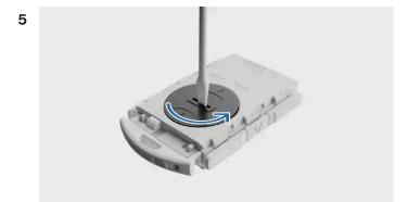
Using a suitable tool, such as a screwdriver or a coin, turn the battery cover counter-clockwise to release it.
