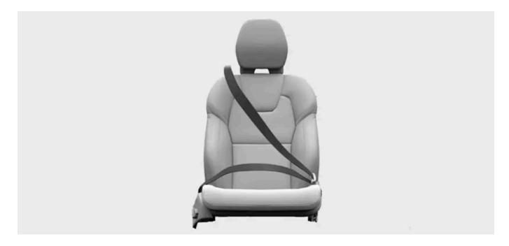
The seat belt locks itself to act as a safety restraint under certain conditions, such as sudden and forceful pulling of the belt, if the vehicle is driven aggressively and if the vehicle is on a steep incline.
