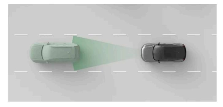
Adaptive cruise control [1] can support you with maintaining a set speed. When driving with adaptive cruise control active, you select a target speed. The vehicle then manages acceleration and braking to meet that target while also adapting to surrounding traffic.
