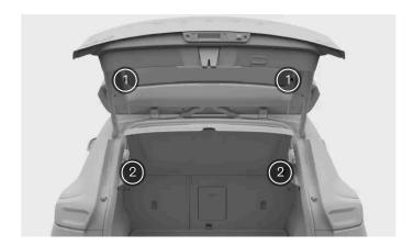
There are two attachment points on the parcel shelf itself and two on the trunk hatch. When the parcel shelf is attached, cords run between attachment points on the parcel shelf and the trunk hatch.
