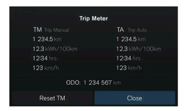
Your vehicle has a trip meter and an odometer. The trip meter can show information on the vehicle's driving distance and time, as well as your average driving speed.
