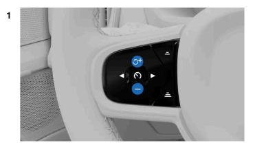
Adjust the target speed using the buttons on the steering wheel.
