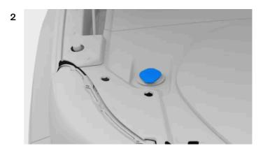
Locate the blue cap with the washer fluid symbol and open it.
