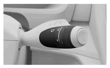
Front wiper controls are on the right-hand steering wheel stalk.
