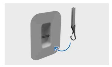
Fastening tether to top tether attachment point
