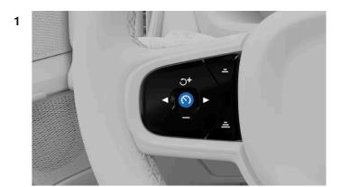
When it's safe to do so, press the adaptive cruise control button (5) on the steering wheel.
