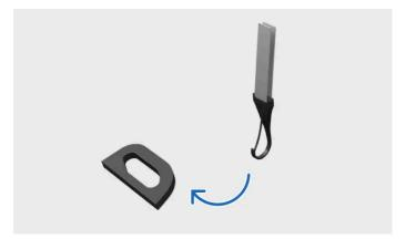
Fastening tether to lower tether attachment point
