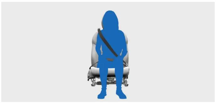
Correctly fastened and adjusted seat belt.
