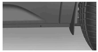
One of the vehicle's four markings showing where the outer lifting points are located.
