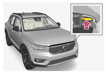
Move the handle under the hood upwards to release the catch and lift the hood.
