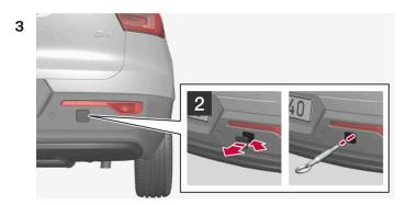
Rear: Remove the cover by placing a coin, key or similar at the mark and prying out the cover.
