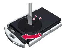
Put the battery cover back into place and turn it clockwise to the CLOSE position.
