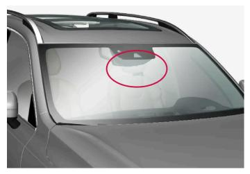
Location of front camera and radar sensor
