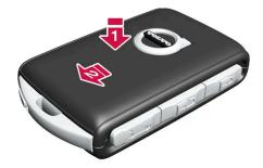
Put the front cover on in the reverse order it was removed. Press the cover down until it clicks and then push it the last few millimeters back to its original position.
