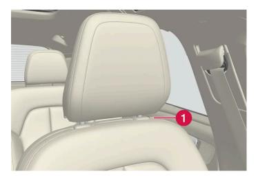
1 The head restraint can be adjusted up or down by pressing the button and manually moving the head restraint to the desired position.
