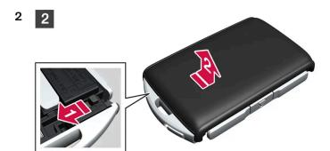
Move the catch behind the front cover to the side and slide the rear cover away from the key ring bracket.
