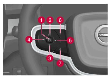
Buttons for speed-controlling functions
