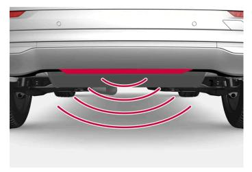
The sensor is located in the center of the bumper.
