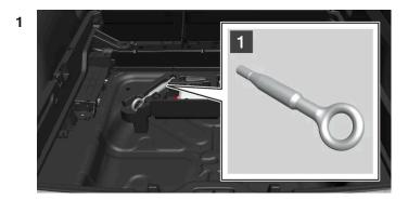
Take out the towing eyelet, which is stored in a foam block under the floor in the cargo compartment.
