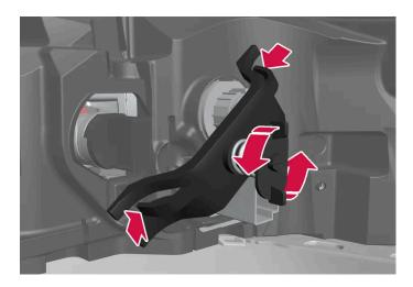
3. Unscrew the spring screw by turning counterclockwise, press the clips into the sides and remove the support bridge. It is simplest to leave one screw in place in the support bridge.
