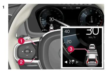
Controls for setting a time interval.
