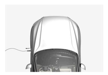
The hybrid battery is recharged using the charging cable. It can also be recharged during light braking and through engine braking in gear position B. The combustion engine can also help recharge the hybrid battery. The vehicle's start battery is charged when the hybrid battery is charged.
