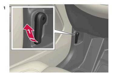
Pull the lever to the side of the pedals to release the hood from its fully closed position.
