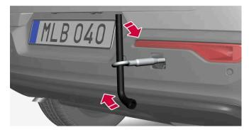
Fasten the eyelet securing by, for example, inserting a lug wrench\* through it and using this as a lever.
