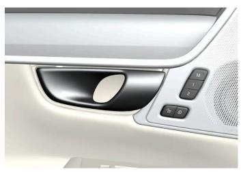
Alternative unlocking method using side door opening handle [1].
