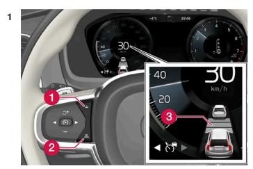
Controls for setting a time interval.
