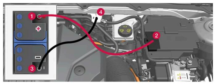
Jumper cable charging points. There are two connecting points under the cover. Only use the one closest to the passenger compartment.
