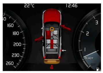
Graphics in the instrument panel with various types of warnings. The warning colors for the doors/tailgate vary depending on the vehicle's speed.
