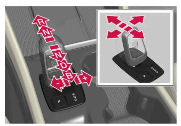
Gear selector and gear selector positions overview.
