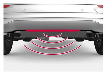
The sensor is located in the center of the bumper.
