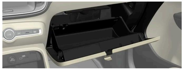
Glove compartment with fold-out hook.
