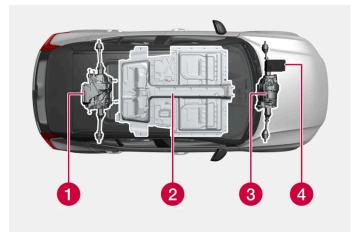
1 Electric motor – The vehicle's electric motor powers the vehicle and regenerates braking energy into electric current.
