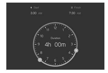
Select Charging - Set timer in the center display and then activate the scheduled charging in Schedule charging. Drag the 🛉 and II controls to set start and stop times for charging.
