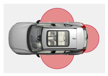
For keyless operation to be possible, the key must be within a distance of about 1 to 1.5 meters (3 to 5 feet) from the vehicle's doors or tailgate.
