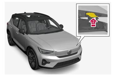
Nove the handle under the hood upwards to release the catch and lift the hood.
