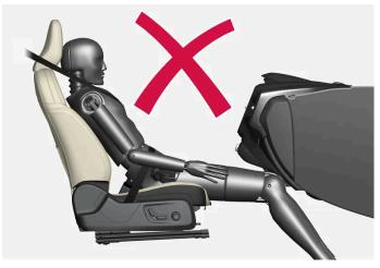
$\label{eq:example} \mbox{Example of incorrect seating position} - \mbox{the passenger must not have slid forward on the seat cushion}.$
