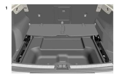
Push the folding cargo compartment floor forward so that it folds together.
