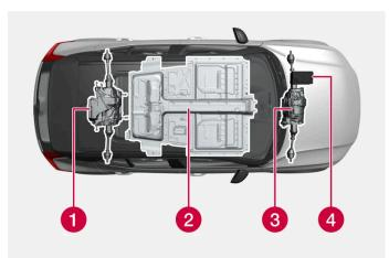
1 Electric motor – The vehicle's electric motor powers the vehicle and regenerates braking energy into electric current.
