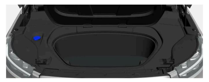
There is additional storage space under the hood. The front cargo compartment also contains the vehicle's towing eyelet and tire sealing system.
