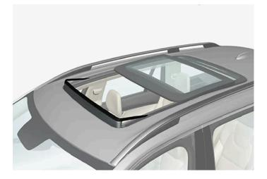
The panoramic roof is equipped with a wind blocker that folds up when the roof is open.
