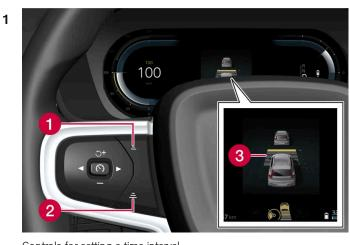
Controls for setting a time interval.
