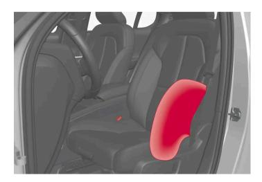
The near-side airbags are located in the front seats' outer backrest frames and help protect the driver and front-seat passenger.
