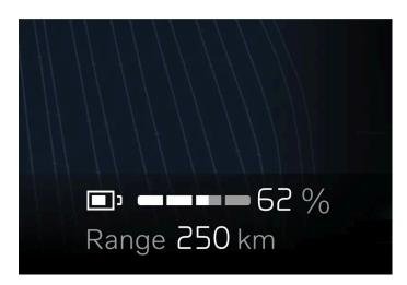
When the vehicle is delivered from the factory, the range is based on the certified value. Once the vehicle has been driven for a while, range is instead based on historical driving patterns.
