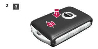
Put the front cover on in the reverse order it was removed. Press the cover down until it clicks and then push it the last few millimeters back to its original position.
