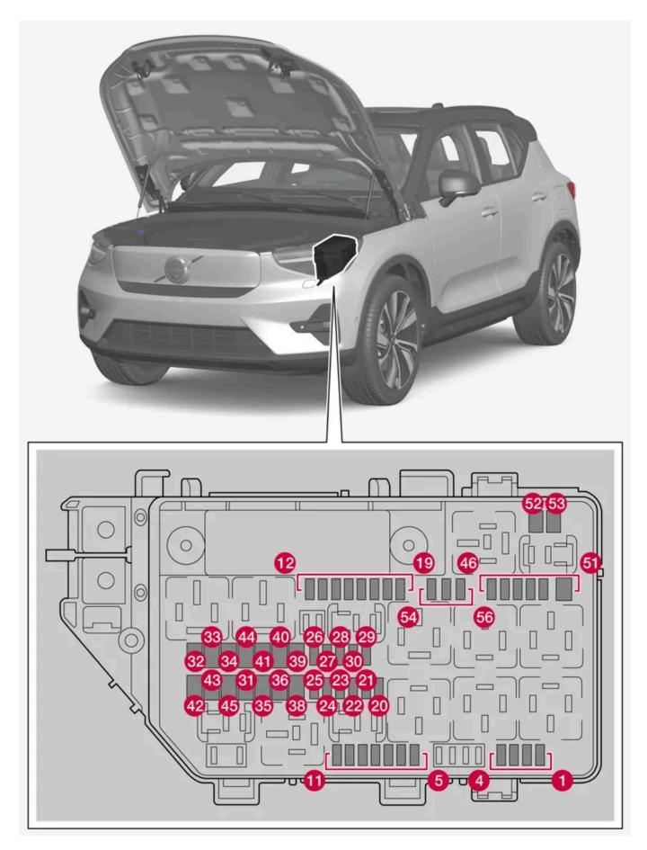
To access fuses under the hood, a number of panels around the storage compartment must be removed.
