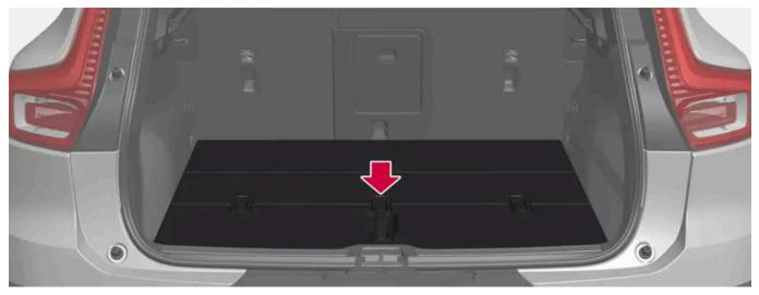
Cargo compartment with storage space under the cargo compartment floor.
