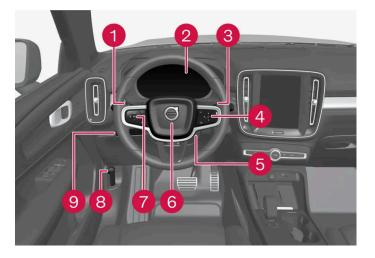
Parking lights, daytime running lights, low beams, high beams, turn signals, front fog lights/cornering illumination\*, rear fog light, trip computer reset
