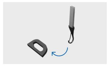
Fastening tether to lower tether attachment point
