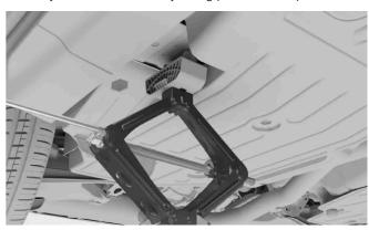
g Raise the vehicle to an appropriate height. Do not raise it higher than necessary for the work you're doing.
