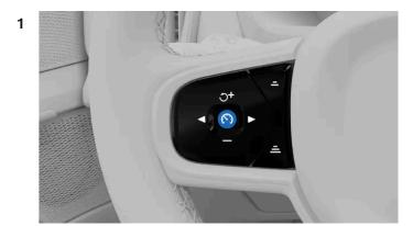
When it's safe to do so, press the Pilot Assist button (5) on the steering wheel.
