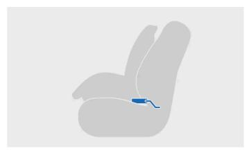
Child restraint installed using ISOFIX<sup>[1]</sup>
