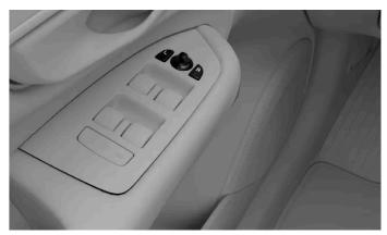
Controls for adjusting the door mirrors
