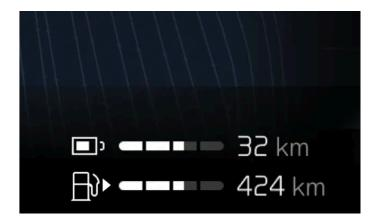
Your range is primarily related to your vehicle's battery, the amount of fuel left in the tank, and your driving practices, but external conditions can also be a factor. The battery level and expected range are displayed in the instrument panel. The expected range is calculated based on your driving pattern, both current and historical.
