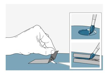
If the damage has not reached all the way down to the metal, then touch-up paint can be applied immediately after the surface has been cleaned.
