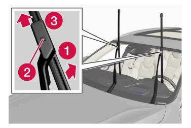
Make sure that the windshield wipers are in service position and raise the wiper blades. Service position is activated/deactivated via the center display when the vehicle is stationary and the windshield wipers are not on.
