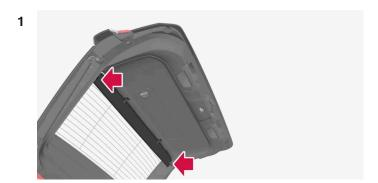
Turn the flap so that the screw side faces down and guide the pin into the bracket on one side of the tailgate.
