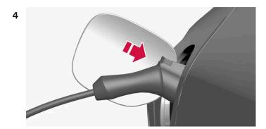
Remove the charging handle's protective cover and push the charging handle all the way into the vehicle's socket.
