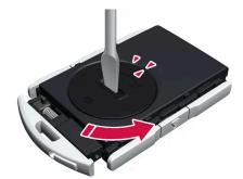
Turn the battery cover counterclockwise to the OPEN position. Use a screwdriver, coin or similar.
