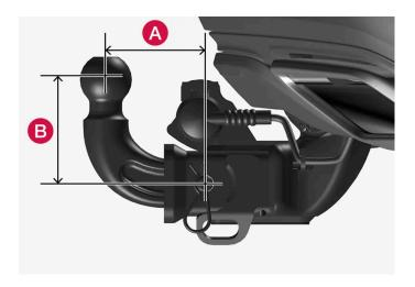
The ball mount must fall within the geometric limits for the towbar, for both distance (A) and height (B). Geometric limits are described on a type plate located on the towbar.
