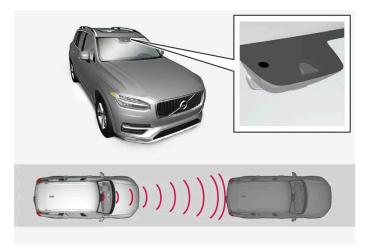
The camera/radar sensor measures the distance to the vehicle ahead.
