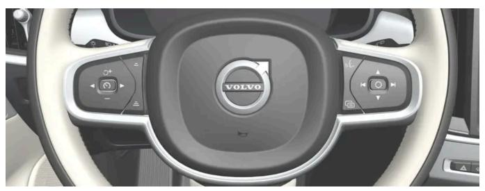
The horn is located in the center of the steering wheel.
