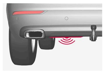
The sensor is located to the left of center under the rear bumper [1].
