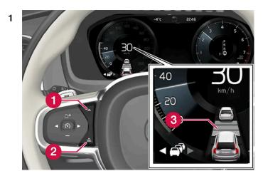
Controls for setting a time interval.
