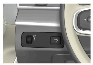
Thumb wheel (to the left) for adjusting interior brightness.
