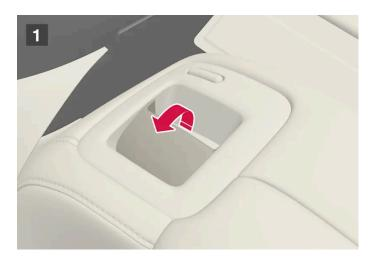
For vehicles with electrically folding\* head restraints, the outboard head restraints can be folded using the handle on the top of the seat (see illustration 1.) Note that this method also folds down the backrests. To fold down only the head restraints, e.g. to improve visibility, use the center display \* instead.
