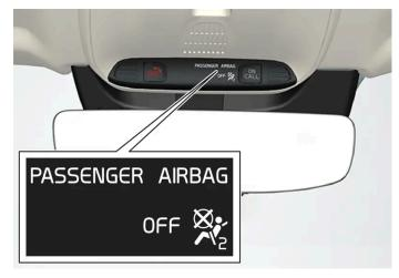
Occupant Weight Sensor (OWS) indicator light
