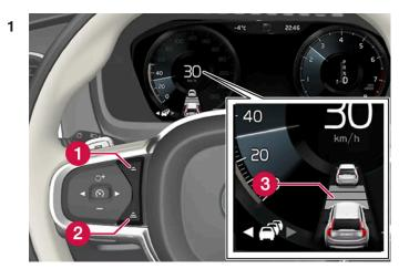
Controls for setting a time interval.
