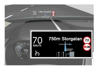
The head-up display presents information that the driver should react to immediately. For example, traffic warnings, speed information and navigation messages\*. Road sign information and incoming phone calls are also shown in the head-up display. These can be handled using the right-side steering wheel keypad or the center display.
