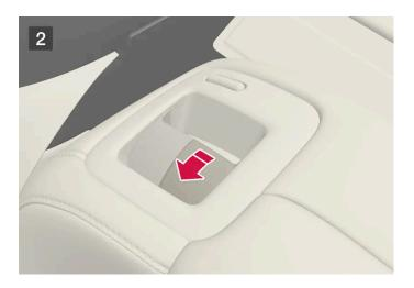
For vehicles without electrically folding backrests, fold the outboard head restraints manually using the inner control on the top of the seat (see illustration 2).
