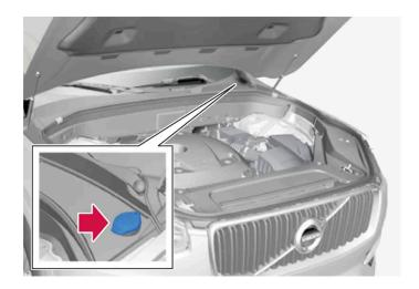
Fill washer fluid into the reservoir with the blue cover. The reservoir is used for the windshield washer, tailgate window washer and headlight washer\*.
