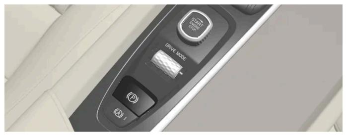
The parking brake controls are located in the tunnel console between the seats.
