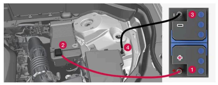
Jumper cable connecting points. Engine compartment appearance may vary depending on vehicle model and equipment level.
