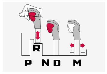
Shiftlock for vehicles with large gear selectors.
