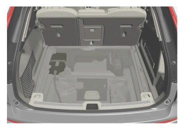
If the vehicle is a mild hybrid, it instead has a 48 V support battery located to the left in the cargo compartment. The 48 V support battery may only be handled by an authorized workshop.
