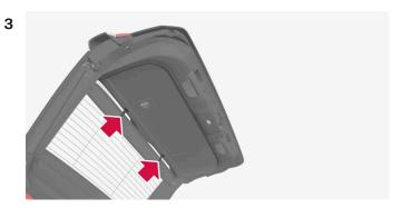
Press the two upper clips in the respective recess in the tailgate so it clicks into place.
