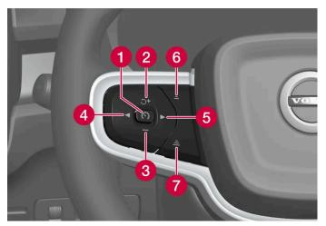
Buttons for speed-controlling functions
