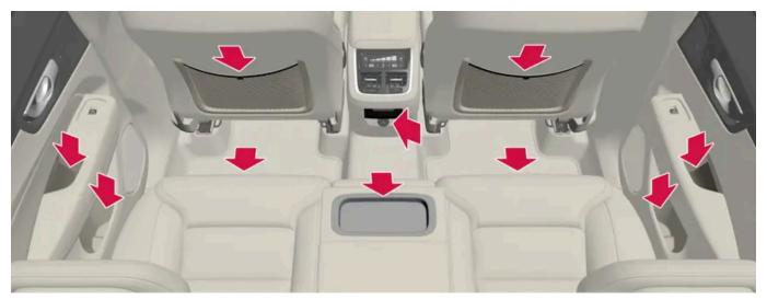
Storage compartment in the door panel, cup holders\* in the center seat's backrest, storage pocket in the front seat's backrest, USB ports in the tunnel console and storage compartment under the seat.
