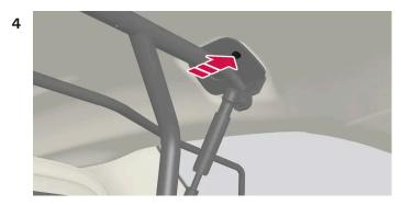
Screw the provided screw into place using the provided 6 mm Allen wrench. Repeat on the other side. Recommended torque: 20 Nm (15 ft-lb).
