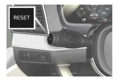
1 Reset all information in trip odometer TM (i.e. mileage, average fuel consumption, average speed and driving time) by pressing and holding the RESET button on the left-hand steering wheel lever.
