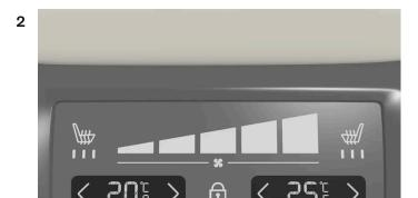
Temperature controls on the rear climate panel of the tunnel console.
