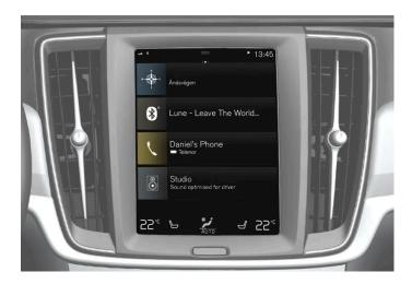
Many of the vehicle's main functions are controlled from the center display, a touchscreen that reacts to taps and other gestures. This minimizes the number of physical buttons and controls needed in the vehicle. The screen can also be operated while wearing gloves.
