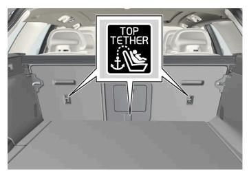
Top tether anchors and symbols on the rear side of the rear seat backrests. There is no symbol for the center anchor position.
