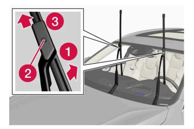
Raise the wiper arms to the service position. Service position is activated/deactivated via the function view in the center display when the car is stationary and the windshield wipers are not on.
