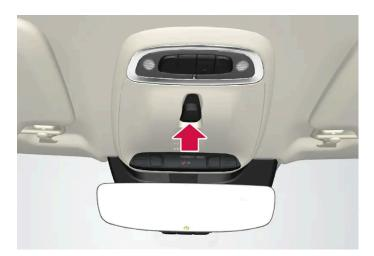
The panoramic roof and sun curtain are operated using the controls in the ceiling.
