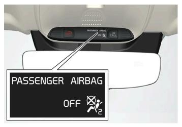
Occupant Weight Sensor (OWS) indicator light
