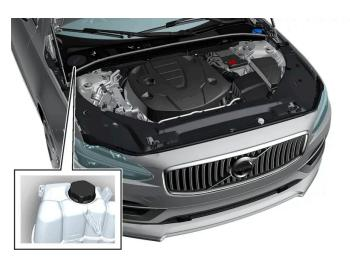
Coolant expansion tank, left-hand drive vehicle.
