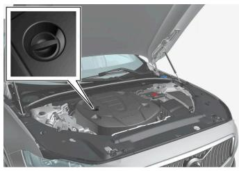
It may be necessary to top up engine oil between regularly scheduled services. No action is necessary with regard to engine oil level until a message appears in the instrument panel.
