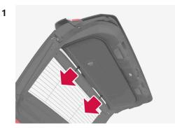
Pull the upper clips of the cover straight out of the tailgate.
