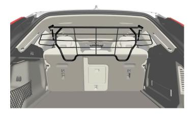
For safety reasons, the steel grid must always be installed and secured correctly.
