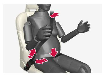
The seat belt should fit closely against the shoulder, with the diagonal section between the breasts and to the side of the stomach.
