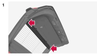
Turn the flap so that the screw side faces down and guide the pin into the bracket on one side of the tailgate.
