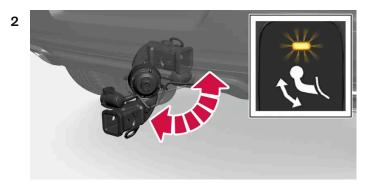
Secure the hitch into position by pushing it back to its retracted position under the bumper, where it will lock into place.
