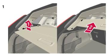
Press the handle section of the cargo compartment slightly upward.
