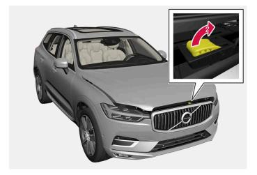
2 Swipe your hand from left to right under the hood, grasp the handle and move it up and to the side to release the catch and lift the hood.
