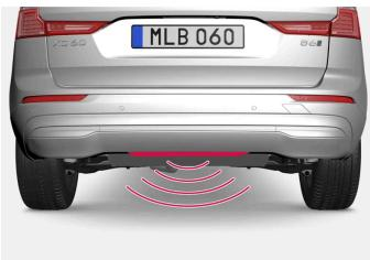
The sensor is located in the center under the bumper.
