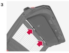
Press the two upper clips in the respective recess in the tailgate so it clicks into place.
