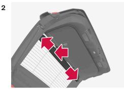
Carefully pull the flap out of the bracket on one side of the tailgate and then the other. If necessary, press the flap together slightly to make it more flexible and facilitate removal.
