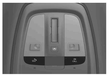
The functions are available via ON CALL and the SOS buttons in the overhead console.
