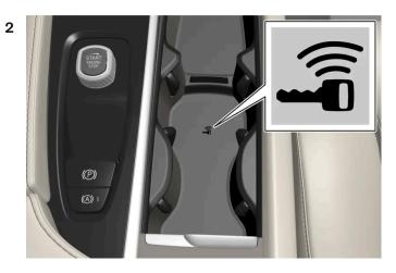
Place the key on the key symbol in the backup reader in the tunnel console's cup holder.
