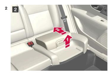
Lift the front edge of the booster cushion and press it rearward toward the backrest to lock it into position.
