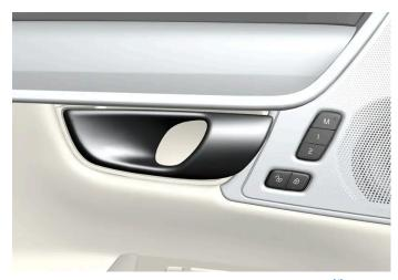
Alternative unlocking method using side door opening handle<sup>[1]</sup>.
