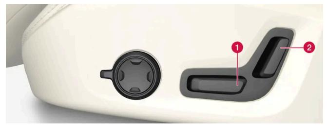
1 Move the passenger seat forward/rearward by moving the control forward/rearward.
