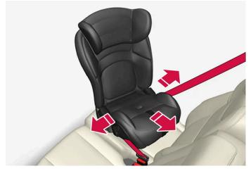
The convertible seat can be removed by unbuckling the seat belt and letting it retract completely.
