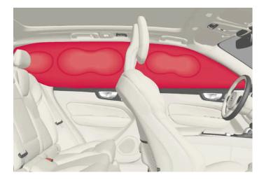
The inflatable curtains are installed along both sides of the inside of the roof and help protect occupants in the vehicle's outer seats. IC AIRBAG is embossed on the panels.
