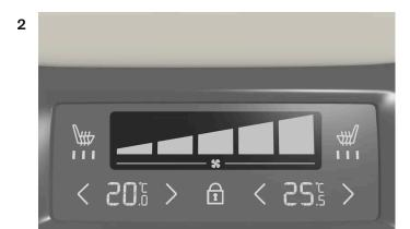
Blower controls on the rear climate panel of the tunnel console.
