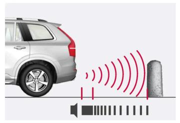
The warning signal has a continuous tone when the obstacle is less than approx. 30 cm (1 foot) from the vehicle.
