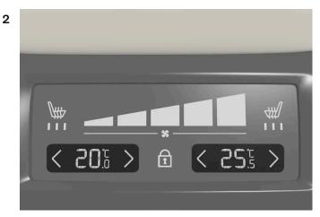
Temperature controls on the rear climate panel of the tunnel console.
