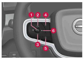
Buttons for speed-controlling functions
