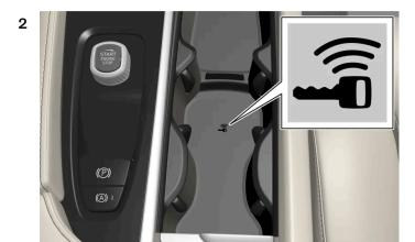
Place the key on the key symbol in the backup reader in the tunnel console's cup holder.
