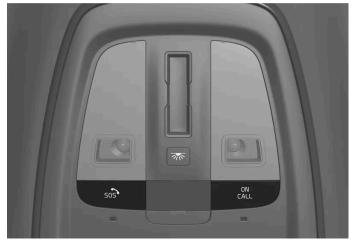
The functions are available via ON CALL and the SOS buttons in the overhead console.
