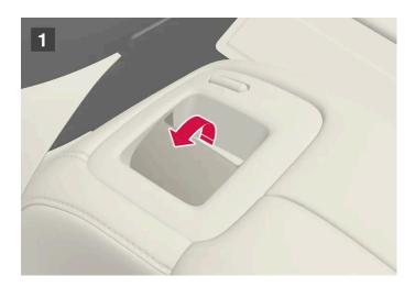
For vehicles with electrically folding \* head restraints, the outboard head restraints can be folded using the handle on the top of the seat (see illustration 1.) Note that this method also folds down the backrests. To fold down only the head restraints, e.g. to improve visibility, use the center display \* instead.
