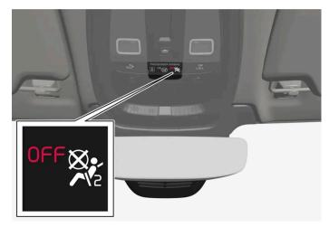
Occupant Weight Sensor (OWS) indicator light
