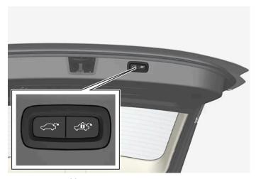
Location of button(s) on underside of tailgate.
