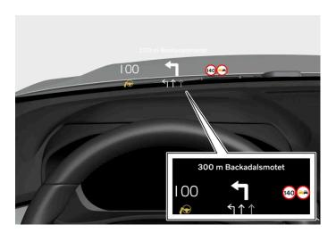
The head-up display projects information from the instrument panel onto the windshield in front of the driver. This information can only be seen from the driver's position.
