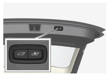
Location of button(s) on underside of tailgate.
