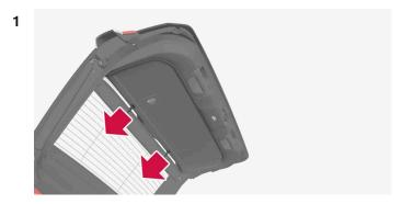
Pull the upper clips of the cover straight out of the tailgate.
