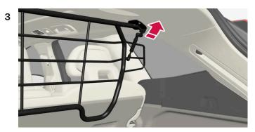
Position the grid's attachment points in the ceiling brackets.
