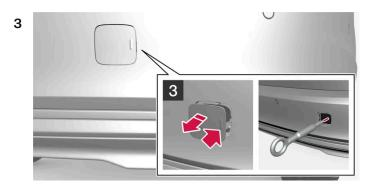
Rear: Remove the cover by pressing on the mark with a finger while folding out the opposite side/corner.
