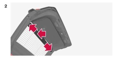
Carefully pull the flap out of the bracket on one side of the tailgate and then the other. If necessary, press the flap together slightly to make it more flexible and facilitate removal.
