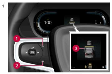
Controls for setting a time interval.
