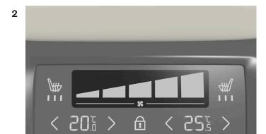
Blower controls on the rear climate panel of the tunnel console.
