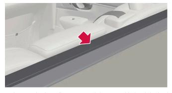
Make sure the front flap is pointed downward behind the backrest before the cassette is put into place.
