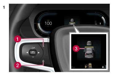
Controls for setting a time interval.
