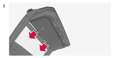
Pull the upper clips of the cover straight out of the tailgate.
