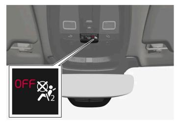
Occupant Weight Sensor (OWS) indicator light
