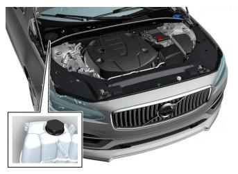
Coolant expansion tank, left-hand drive vehicle.
