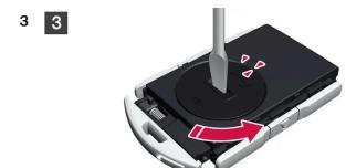
Turn the battery cover counterclockwise to the OPEN position. Use a screwdriver, coin or similar.
