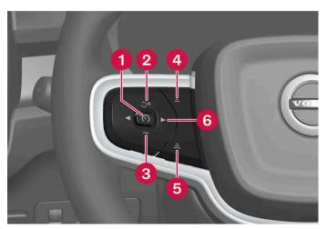
Buttons for speed-controlling functions
