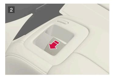
For vehicles without electrically folding backrests, fold the outboard head restraints manually using the inner control on the top of the seat (see illustration 2).
