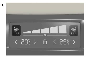
Seat heating controls and indicator lights on the rear side of the tunnel console.
