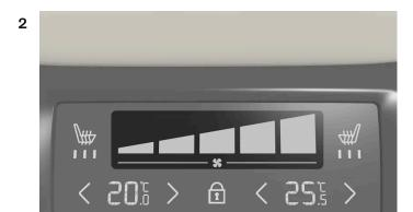
Blower controls on the rear climate panel of the tunnel console.
