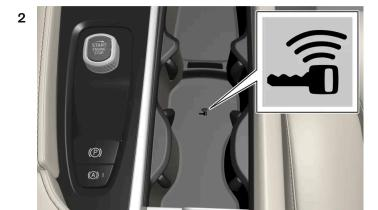
Place the key on the key symbol in the backup reader in the tunnel console's cup holder.
