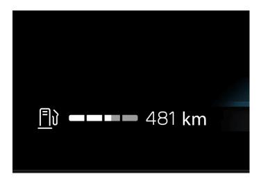
The white area in the fuel gauge indicates the amount of fuel left in the tank.
