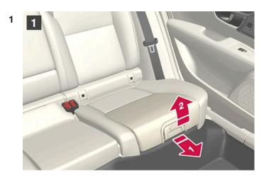
1 Pull the handle forward and upward to release the booster cushion.
