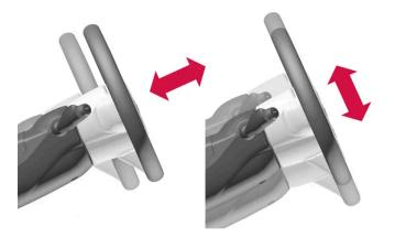
The steering wheel's reach and height can be adjusted.
