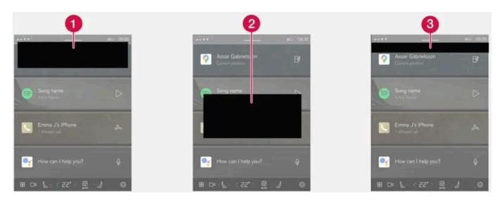
1 Shown at the top of the center display. Requires immediate action and may have up to three buttons allowing the user to manage the message. Dismiss by swiping right or left. The message will then be saved in Notifications view.
