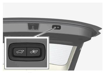
Location of button(s) on underside of tailgate.
