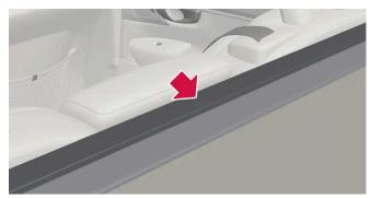
Make sure the front flap is pointed downward behind the backrest before the cassette is put into place.
