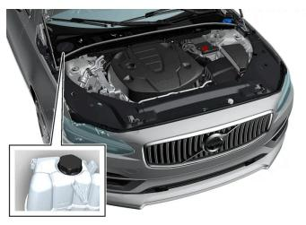
Coolant expansion tank, left-hand drive vehicle.
