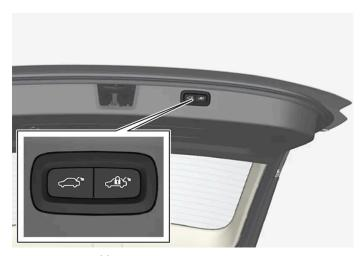
Location of button(s) on underside of tailgate.
