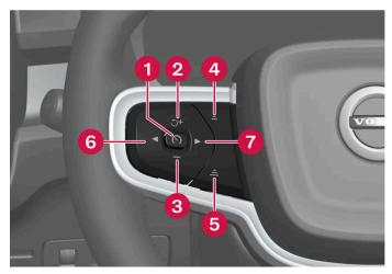
Buttons for speed-controlling functions
