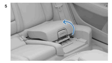
Lift the child seat upwards by the front end and push it back against the backrest.
