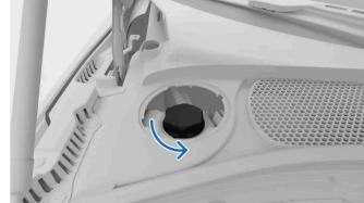
Unscrew the coolant reservoir cap.
