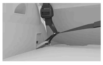
7 Tighten the straps to make the safety net tight and more secure.
