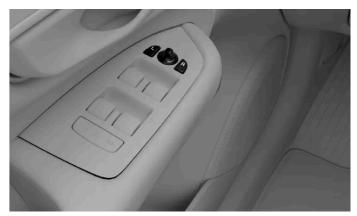
Controls for adjusting the door mirrors
