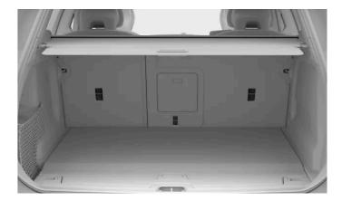
The top tether attachment point locations for the outer rear seats are indicated by the top tether symbol.
