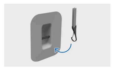
Fastening tether to top tether attachment point
