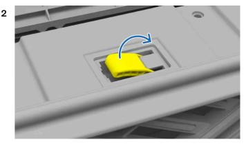
Locate the second lever below the front edge of the hood and pull it to the right.
