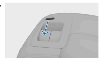
Pull the handle on the seat backrest. A red indicator near the backrest lock indicates that the backrest is no longer locked.
