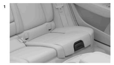
Pull the handle on the front of the seat cushion to release the lock.
