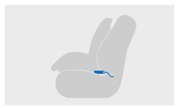
Child restraint installed using ISOFIX<sup>[1]</sup>
