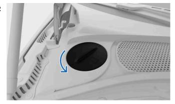
Open the panel hatch in the upper-left corner of the engine compartment to access the coolant container.
