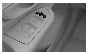
Controls for adjusting the door mirrors
