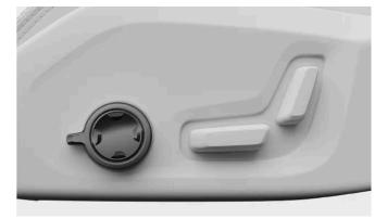
The seat adjustment knob is located on the side of the seat closest to the door.
