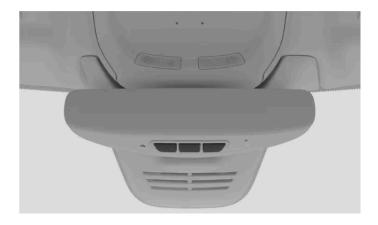
HomeLink is integrated in the rearview mirror and consists of three buttons and an indicator light. You can connect one device per button. You can add, change or delete a connection to a device.
