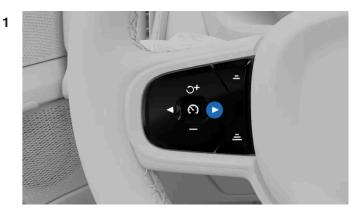
Press the switch button  $\blacktriangleright$  on the steering wheel.
