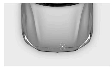
The second lever is below the front edge of the hood, on the driver's side.
