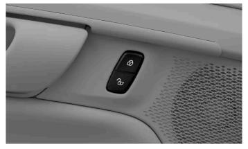
The central lock can be controlled from the front seats using the buttons on each respective door.
