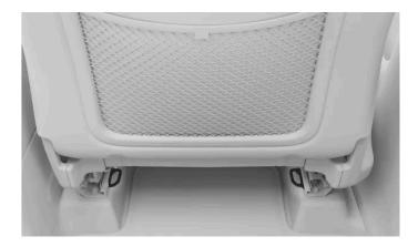
The lower tether attachment points can be found at the back of the floor rails of the front seats.
