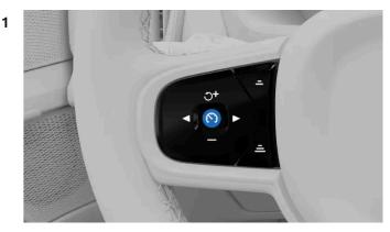
When it's safe to do so, press the Pilot Assist button  $\mathfrak{O}$  on the steering wheel.
