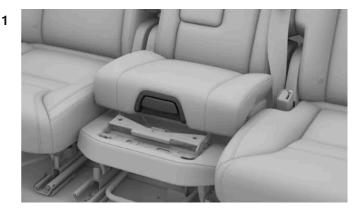
Pull the handle on the front of the child seat to release the lock.
