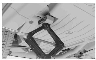
g Raise the vehicle to an appropriate height. Do not raise it higher than necessary for the work you're doing.
