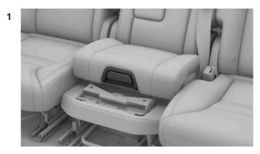
Pull the handle on the front of the child seat to release the lock.
