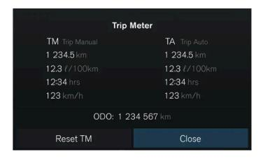
Your vehicle has a trip meter and an odometer. The trip meter can show information on the vehicle's driving distance and time, as well as your average fuel consumption and driving speed.
