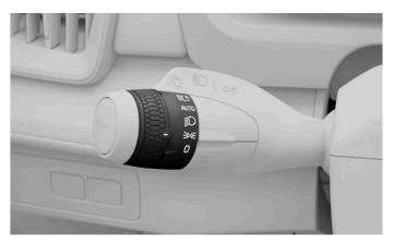
The position lights symbol on the rotating ring on the left-hand stalk
