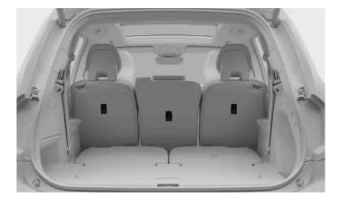
The top tether attachment point locations for the outer second-row seats are indicated by the top tether symbol.
