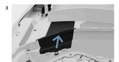
Open the hatch lock and lift the hatch upward to release it.
