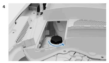
Unscrew the coolant reservoir cap.
