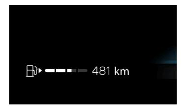
The instrument panel shows the fuel gauge at all times.
