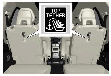
Six-seat models: Top tether anchors and symbols on the rear side of the second row backrests.
