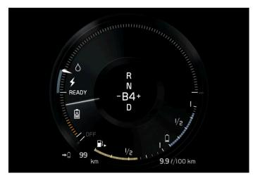
The vehicle is generating current to recharge the battery, e.g. during light braking or engine braking on a downslope.
