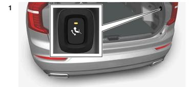
Open the tailgate. There is a button for operating the hitch on the right-hand side at the rear of the cargo compartment. Steady orange illumination from the indicator light in the button shows that the folding function is active.
