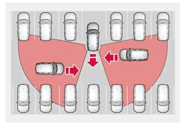
Examples of areas in which Cross Traffic Alert can help the driver detect obstacles while backing up.
