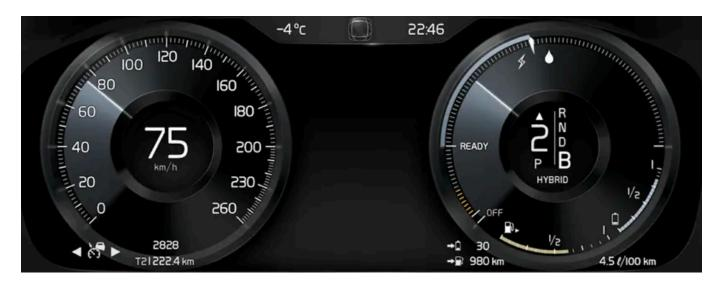
The instrument panel displays information such as speed, incoming phone calls or the track currently playing. It is controlled using the steering wheel keypads.
