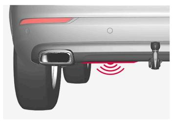
The sensor is located to the left of center under the rear bumper<sup>[1]</sup>.
