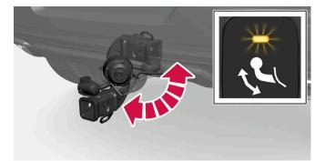
The hitch will fold out and down to an unlocked position – the indicator lamp will flash orange. The hitch is ready to be moved to the locked position.
