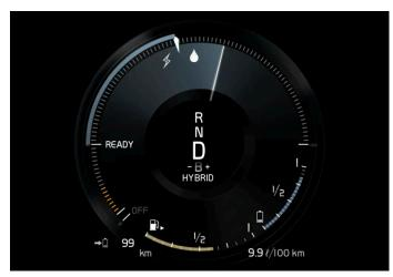
The electric motor cannot supply the requested power and the internal combustion engine will start.
