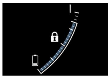
The f symbol is displayed in the hybrid battery gauge when Hold is activated.
