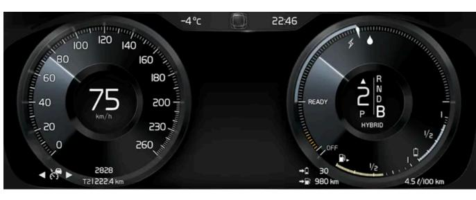
The instrument panel displays information such as speed, incoming phone calls or the track currently playing. It is controlled using the steering wheel keypads.
