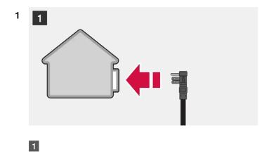
Plug the charging cable into a 120/240 V outlet. Never use an extension cord.
