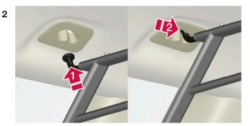
Press one of the grid's hooks into the larger hole in the ceiling attachment point (1). Grasp the grid near the hook and pull/push it into the smaller hole (2).
