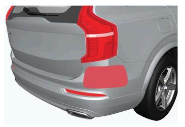
Keep the marked area clean (on both the left and right sides of the vehicle)<sup>[2]</sup>.
