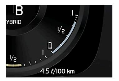
When the vehicle leaves the factory, or after a factory reset, range is based on the certified value.
