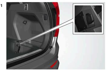
Insert a personal SIM card in the holder. Note that the vehicle's card reader requires **mini SIM** cards.
