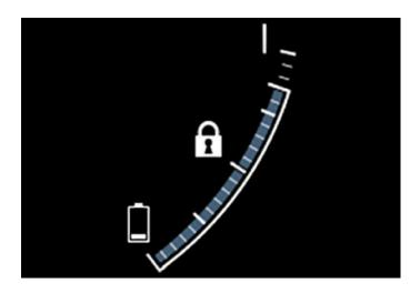
The **f** symbol in the hybrid battery gauge indicates that the **Hold** function is activated. The **f** symbol indicates that the **Charge** function is activated.
