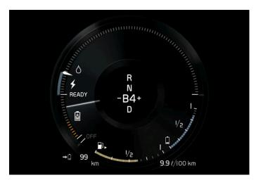
When the battery is being charged with the electric motor braking function, this will be indicated in the instrument panel.
