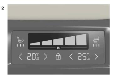
Tap the unlock button on the tunnel console's climate panel to access the controls. 1
