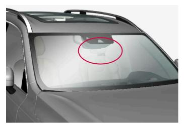
Location of front camera and radar sensor
