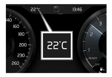
If the vehicle has been stationary, the sensor reading may be higher than the actual temperature.
