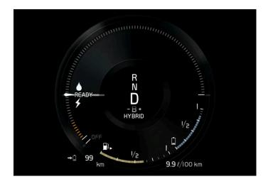
The hybrid gauge shows the ratio between the electric motor's current power consumption and the remaining available power. This information is shown in various ways.
