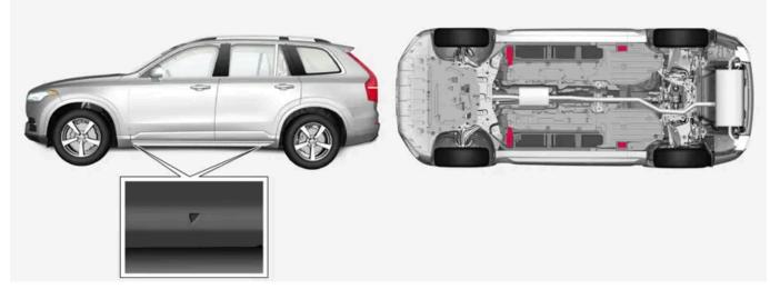
The triangles in the plastic covering indicate where the jack attachment points/lifting points (red areas) are located.
