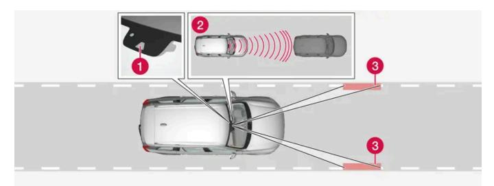
The camera/radar sensor monitors the distance to the vehicle ahead and detects lane markings.
