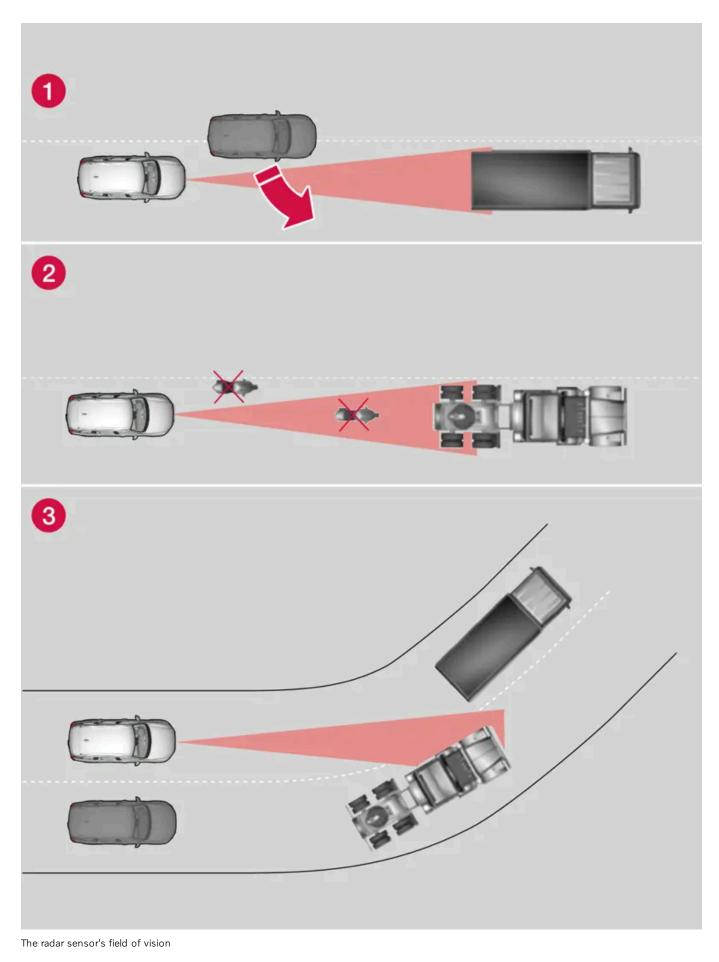
በ The radar sensor's detection of vehicles very close to your vehicle may be delayed in certain situations, e.g. if a vehicle pulls in between your vehicle and the vehicle directly ahead.
