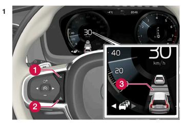
Controls for setting a time interval.
