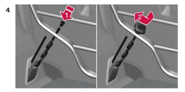
Attach the mounting bracket's hook through the cargo anchoring eyelet near the floor of the cargo compartment and insert the threaded section of the bracket through the grid's lower attachment hole (1).
