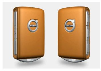
A maximum vehicle speed can be defined for a Care Key. Otherwise, the Red Key functions in the same way as a standard remote key.
