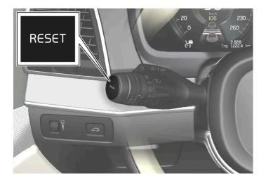
Reset all information in trip odometer TM (i.e. mileage, average fuel consumption, average speed and driving time) by 1 pressing and holding the RESET button on the left-hand steering wheel lever.
