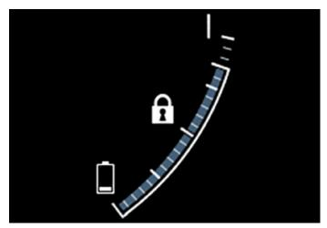
The ft symbol is displayed in the hybrid battery gauge when Hold is activated.
