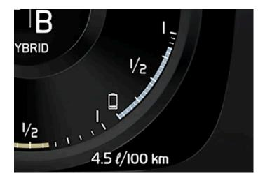
The current in the hybrid battery is used to power the electric motor, but can also be used to heat or cool the vehicle. The trip computer calculates an approximate driving distance with the remaining current in the hybrid battery.
