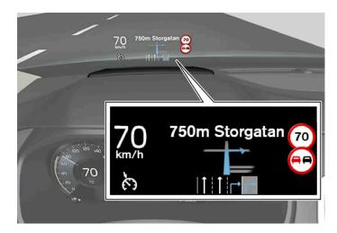
The head-up display presents information that the driver should react to immediately. For example, traffic warnings, speed information and navigation messages\*. Road sign information and incoming phone calls are also shown in the head-up display. These can be handled using the right-side steering wheel keypad or the center display.
