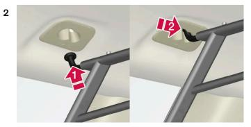
Press one of the grid's hooks into the larger hole in the ceiling attachment point (1).
