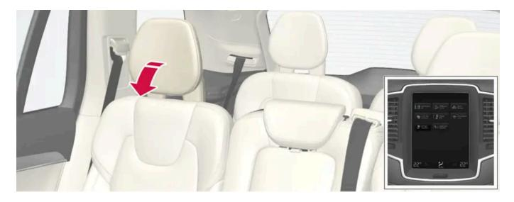
The outer head restraints can be folded via the center display's function view. The head restraint can be folded down when the vehicle is in ignition mode 0.
