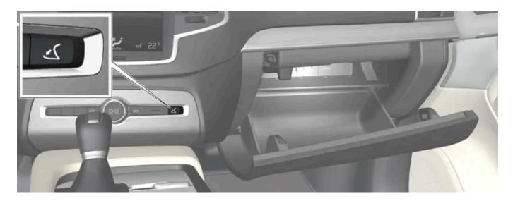
The glove compartment is opened by pressing the opening button in the center console.
