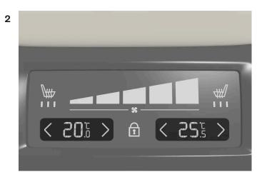
1 Tap the unlock button on the tunnel console's climate panel to access the controls.
