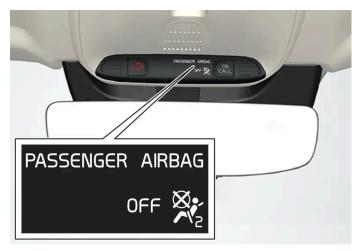
Occupant Weight Sensor (OWS) indicator light
