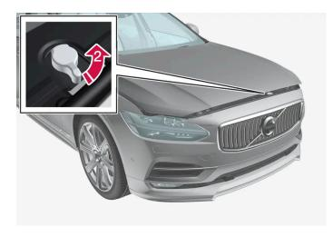
2 Turn the handle under the front edge of the hood counterclockwise to release the catch and lift the hood.
