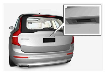
The tailgate is held closed by an electronic locking mechanism.
