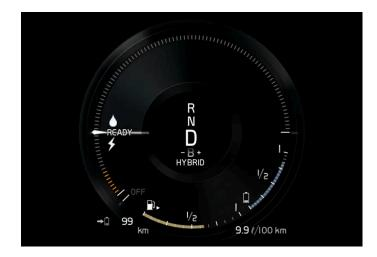
The vehicle has been started, but is stationary and no power is being requested.
