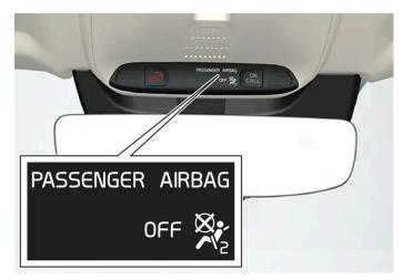
Occupant Weight Sensor (OWS) indicator light
