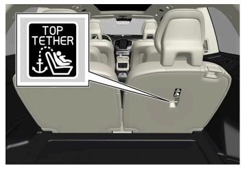
Six-seat models: Top tether anchor and symbol on the rear side of the third row backrests.
