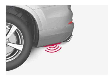
To activate opening and closing using a foot movement on a vehicle with skid plate, make a kicking motion from the side of the vehicle. One of the vehicle's remote keys must be within range (approx. 1 meter (3 feet)) for opening and closing to be possible.
