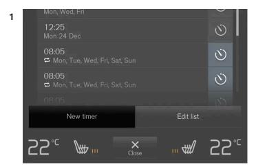
Button for adding a timer setting in the Parking climate tab in Climate view.
