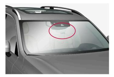
Location of front camera and radar sensor
