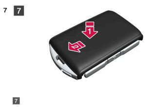
Put the rear cover back into position and press it down until it clicks into place.
