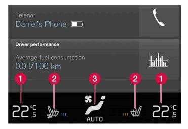
1 Temperature controls for driver and passenger side.
