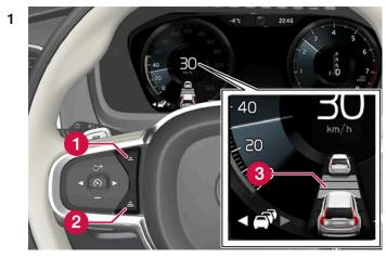
Controls for setting a time interval.
